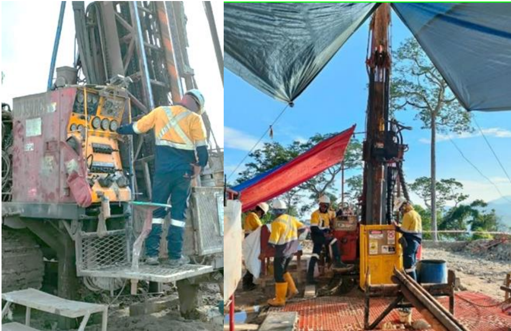
Figure 14: RC (left) and DD (right) drilling at the Wetar Project
