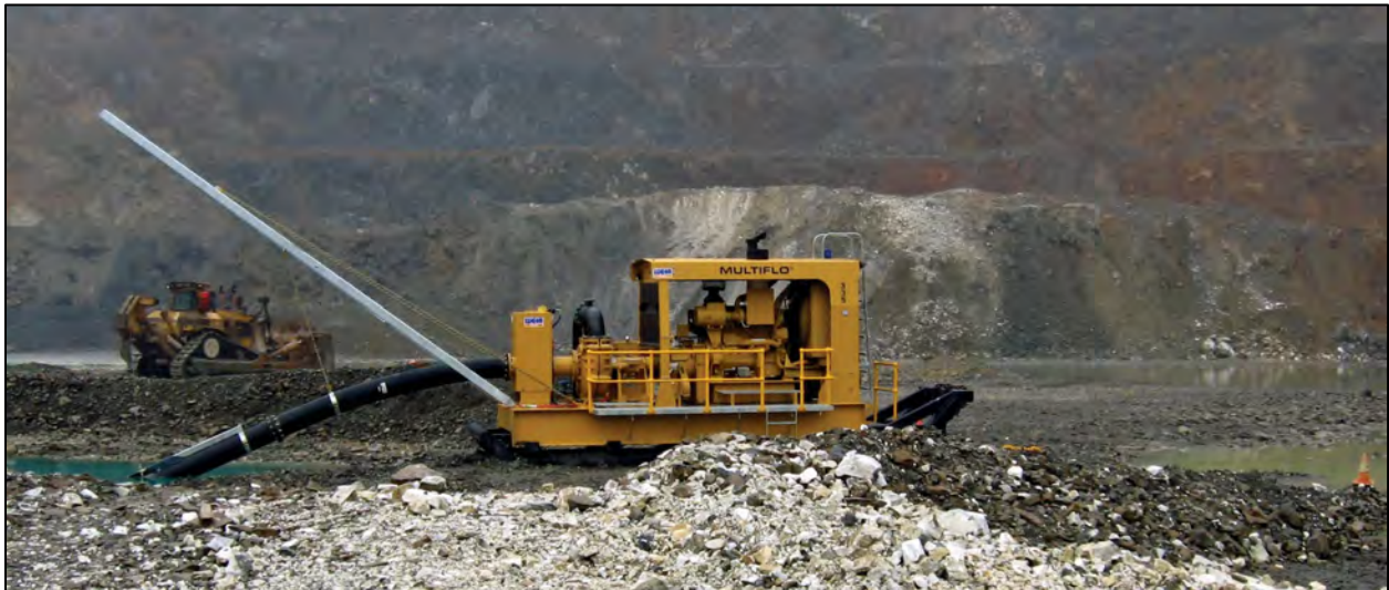
Figure 16-22: Typical Self-Prime Diesel Pump for Pit Sump
