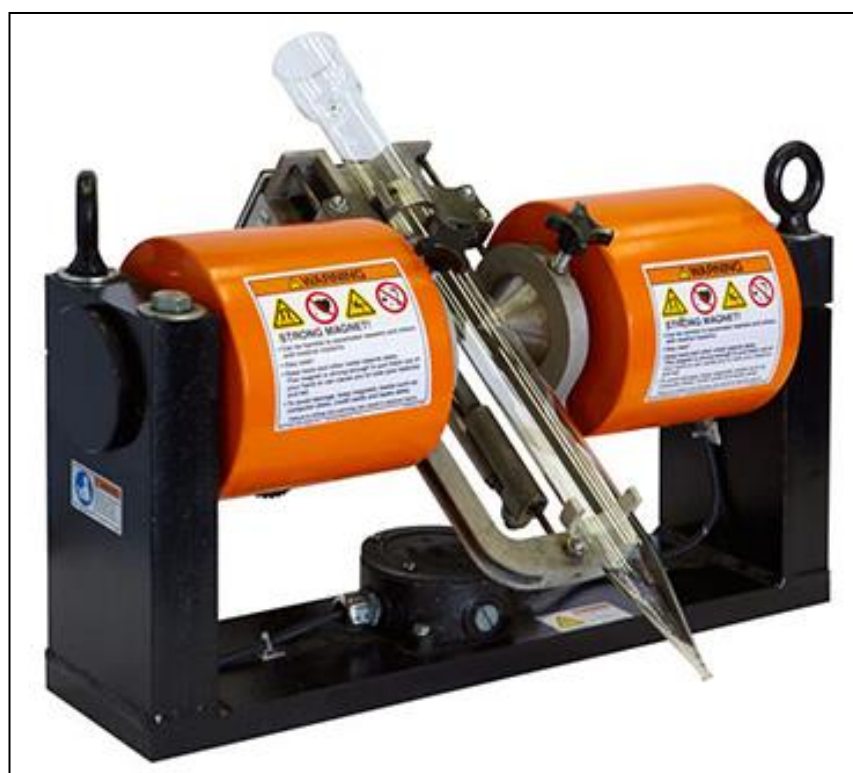
Figure 11-1: A Davis Tube Magnetic Separator
