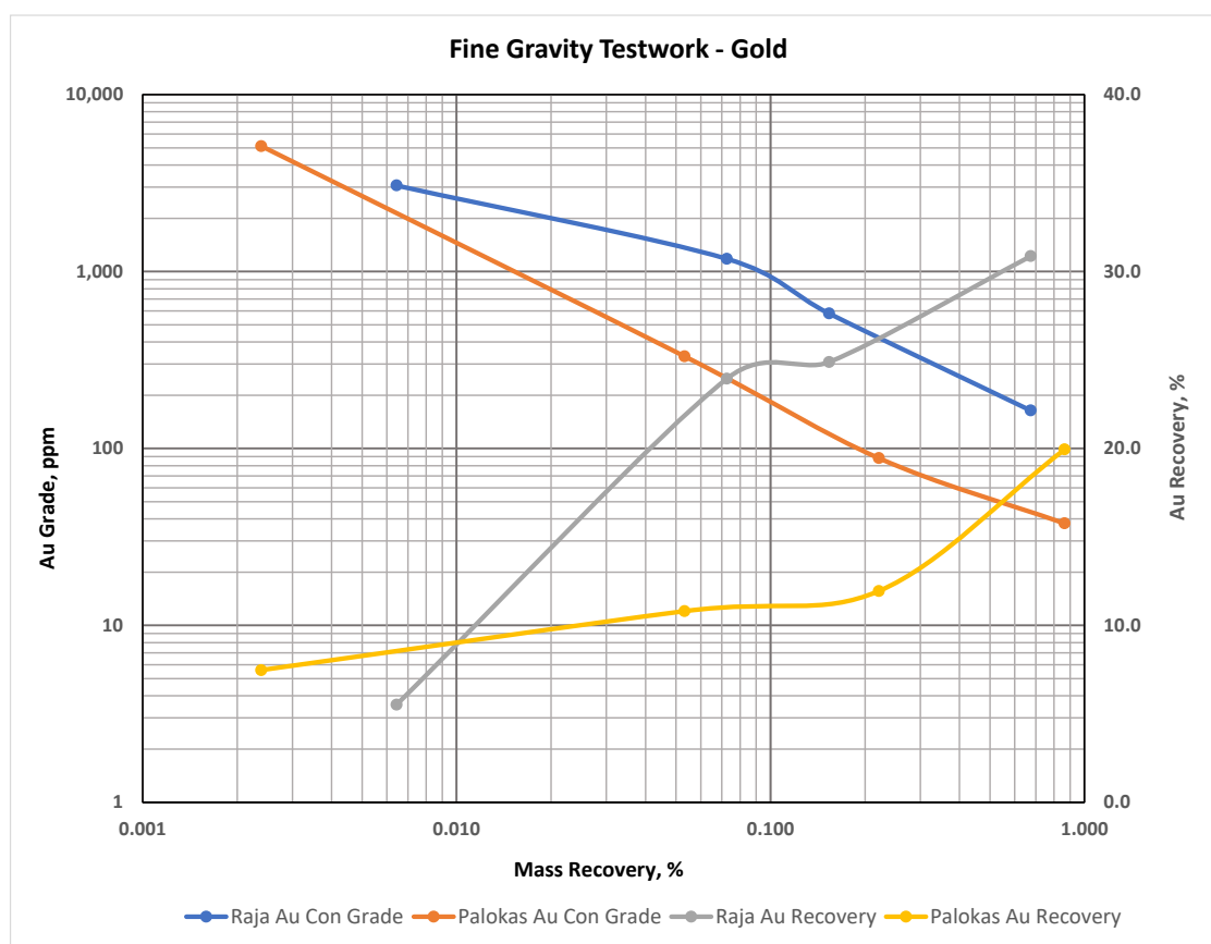
Figure 13-5: Fine gravity testwork results for Raja-South Palokas and Palokas
