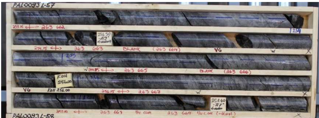
Figure 10-2: Example of marked up drill core tray prior to cutting (PAL0093, core tray 57)
