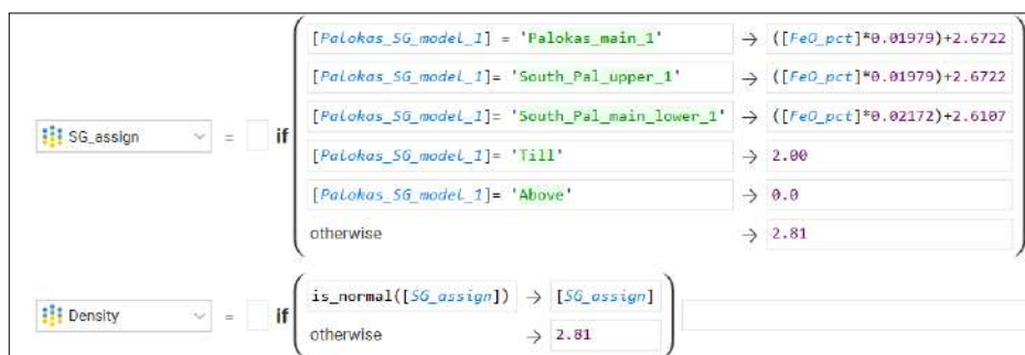
Figure 14-32: Example of density calculations used in block models (image from Leapfrog Edge)
