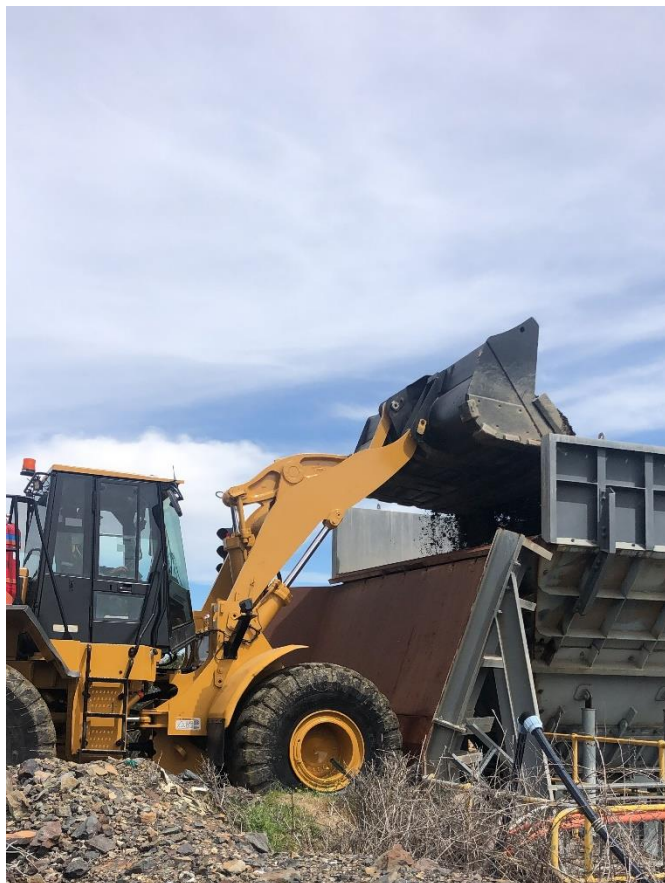
Figure 3 Feeding the primary crusher
