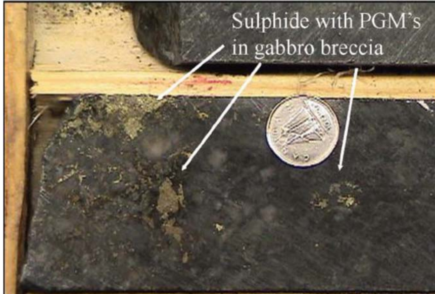
FIGURE 7.16 SULPHIDE MINERALS IN RIVER VALLEY DRILL CORE
