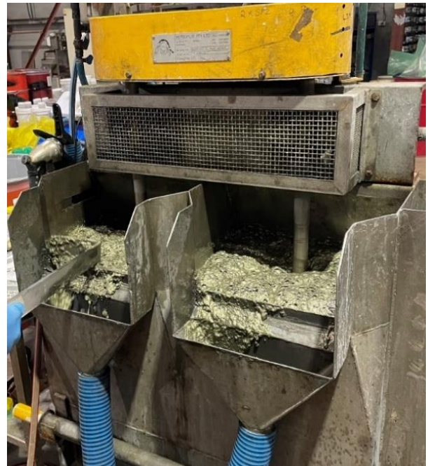
Figure 15: Bulk Concentrate by Flotation
