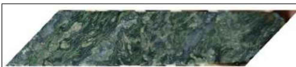
Figure 7.30 Example of ‘Felsic’ Intercalations within the Central Komatiite Zone. Vibrant green fuchsitic wisps are locally developed at the unit boundaries, and are interpreted as selectively replaced, sheared siltstone.
