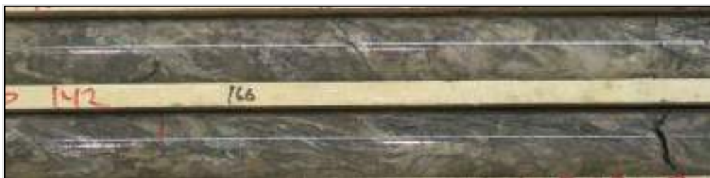
Figure 7.11 Example of Chaotically Veined, Stockwork-like Siderite ± Chlorite ± Sulphide Veins in Altered Mafic-ultramafic Rock with Strong Sericite-Silica Overprint
