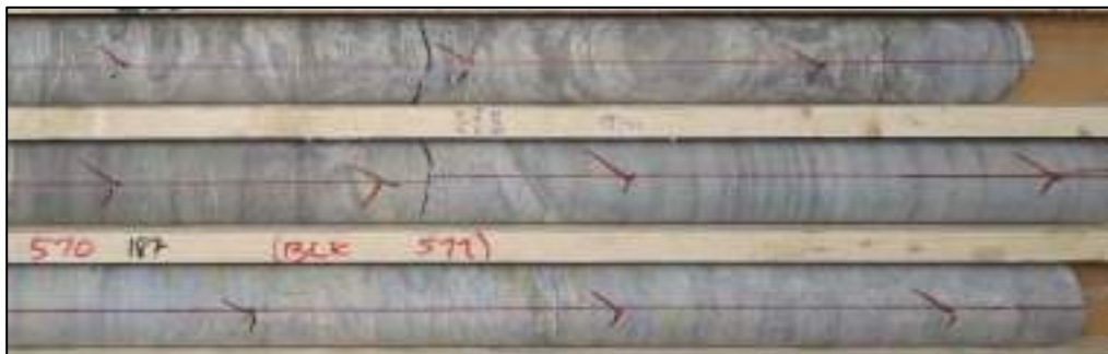
Note: Albite altered meta-siltstone – Hole 121117 at 187 m. *Core size NQ (50.7 mm core width) for all images.
