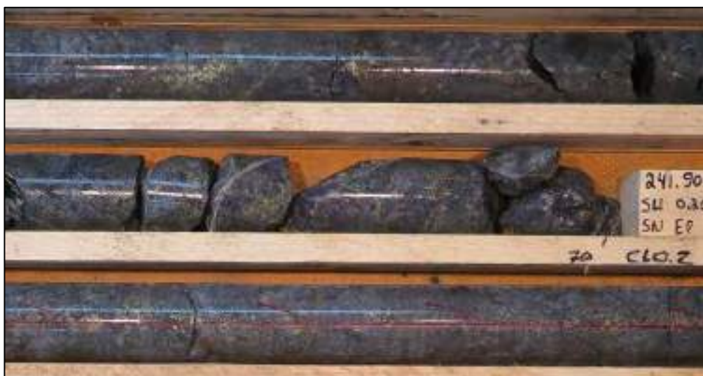
Figure 7.38 Example of Chalcopyrite Filling Narrow, Stringer Like Cracks in Brecciated Vein and Possible Veinlets Within the Quartz-albite-carbonate Brecciated Vein. Where Larger areas of Sulphide Cement Occur Between the Vein Clasts the Dominant Cement is Pyrrhotite
