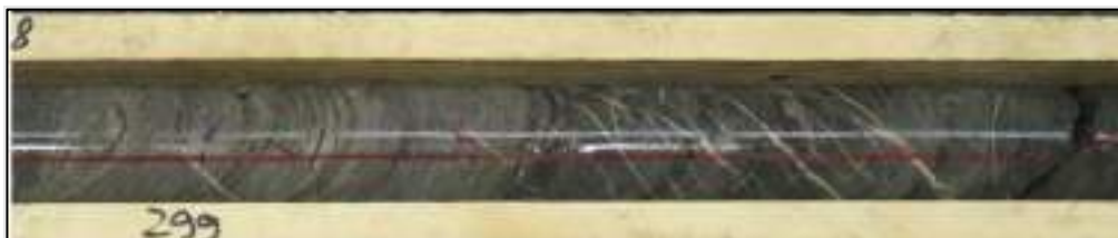
Figure 7.19 Example of Narrow, Late Calcite Veins Cross-Cutting Breccia Development (left) and Sedimentary Banding (right)
