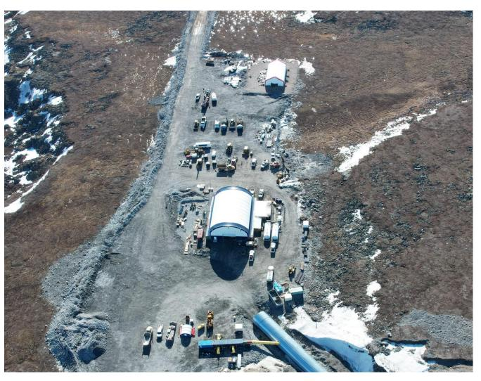
UG work-shop, UG ramp, fuel tank and laydown pads
