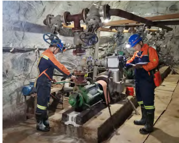
Electromechanics Department of the TLP Mine upgrades the main pumping station with the automatic control system
