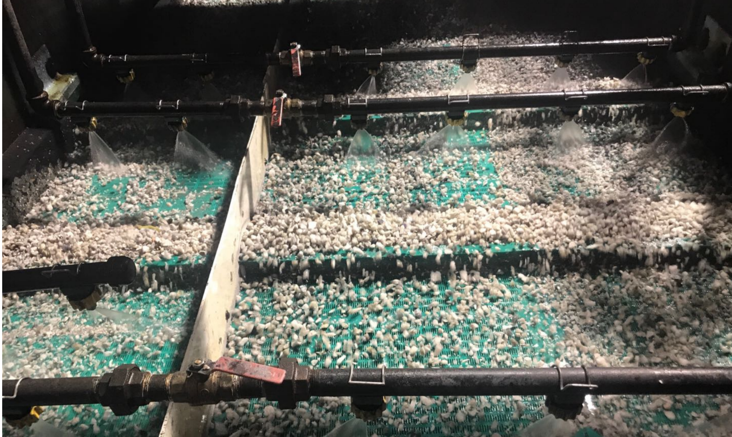
Dense medium beneficiation system (DMS) load test
