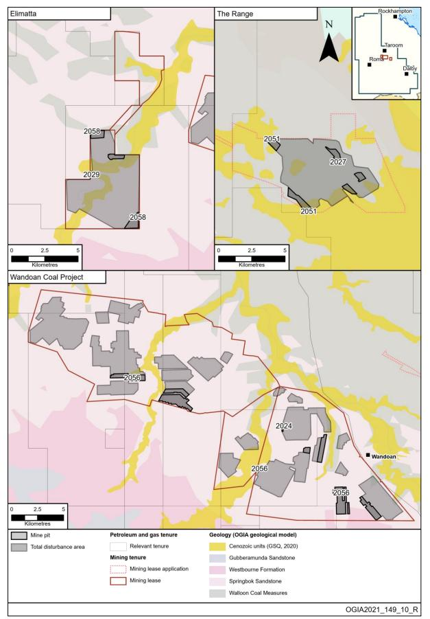
Figure 4-2: Planned coal mining in the Northern Coal Area
