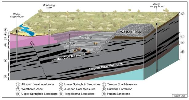
Figure 2-1: Schematic showing the typical profile of an open-cut coal mine at various stages of development
