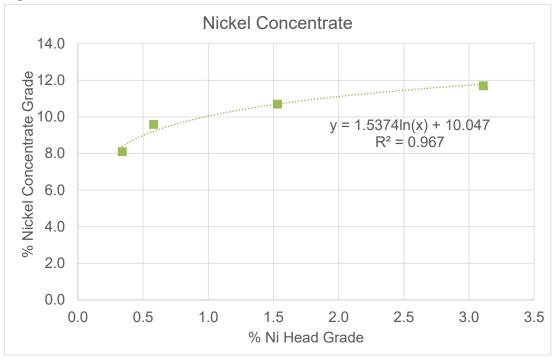
Figure 13.13: Ni Concentrate Grade vs Ni Head Grade
