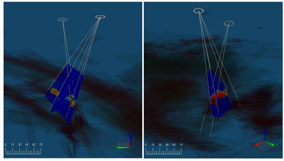
Note: The slowing anomalies, shown in red, correspond very well to the Massive Sulphides and modelled BHEM plates of the CGO West mineralization.
