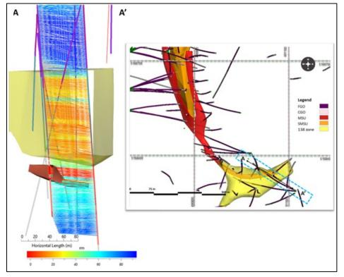
Note: Rays that exhibit maximum attenuation appear red on this image, while weaker attenuation appears as rays coloured from yellow to blue. Two intercepts of massive sulphide mineralization in hole 12TK0153 that are 12.2 m and 2.5 m in thickness appear clearly in this image as two distinct zones of maximum attenuation, while the known semi-massive sulphides of the 138 Zone appear as a cloud of yellow, partially attenuated rays.
