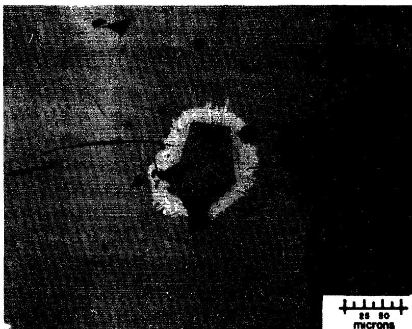
Figure 5: Crystal of uraninite embedded in magnetite and rimmed by hematite from Kenoran granite pegmatite. Byberg occurrence at Hawk Lake [15], Kenora-Dryden area, Ontario.
