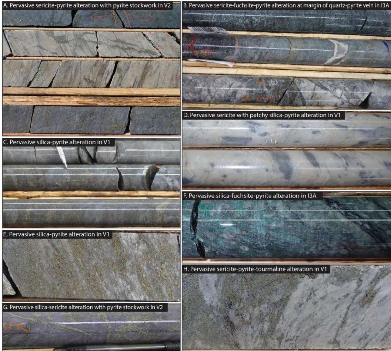
Figure 7-3: Examples of the proximal alteration assemblages observed in drill core at the Windfall deposit V1 = felsic volcanics; V2 = intermediate volcanics; I3A = gabbro intrusion
