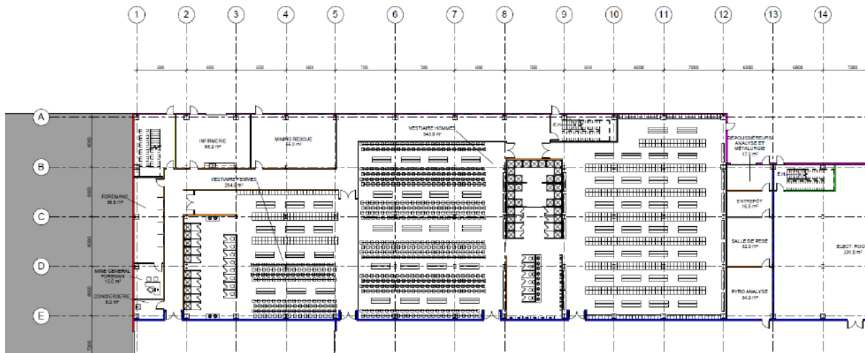
Figure 18-10: Plan view of the mine and process dry layout
