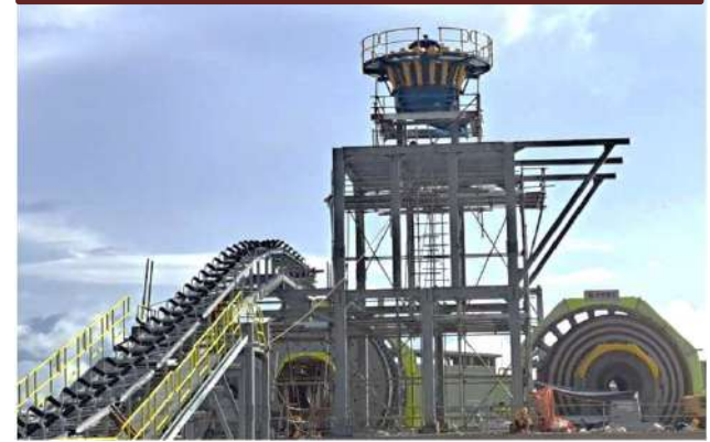
Conveyor to feed ores from crusher to milling unit
