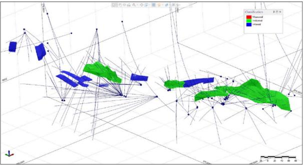
Figure 14-59 Mineral Resource classification for Gamma deposit
