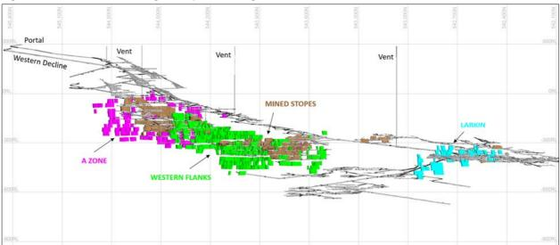
Figure 16-1 Beta Hunt Underground plan looking east
