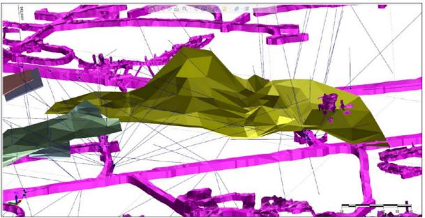
Figure 14-49 B30C\_Ni\_04 lens intersected by underground workings, oblique view
