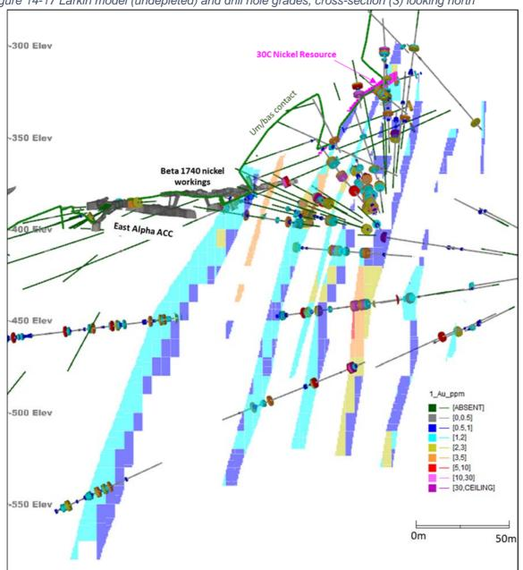
Figure 14-17 Larkin model (undepleted) and drill hole grades, cross-section (3) looking north
