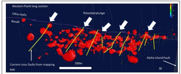
Figure 7-12 Western Flank long section looking northeast - potential ore shoot geometrySource: Karora
