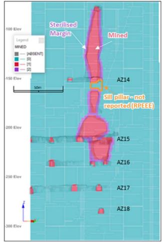
At Larkin, individual blocks that had estimated gold grades greater than the 1.4 g/t, but which were isolated spatially from the main mineralised zones, were not included in the reported Mineral Resource. An example long-section of Zone 140 at Larkin is shown in Figure 14-21.
