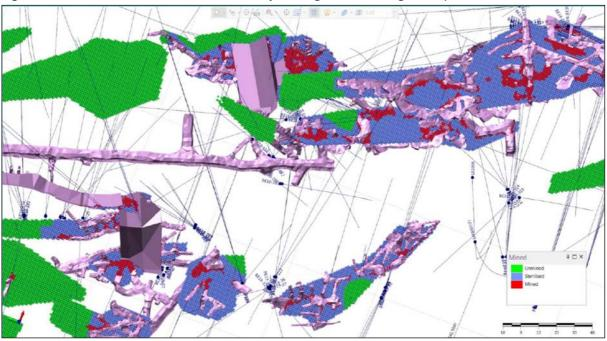
Figure 14-47 Beta Central lodes intersected by underground workings, oblique view
