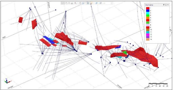
Figure 14-32 Oblique View of the B30 and B40 Domains Used for Geostatistical Analysis
