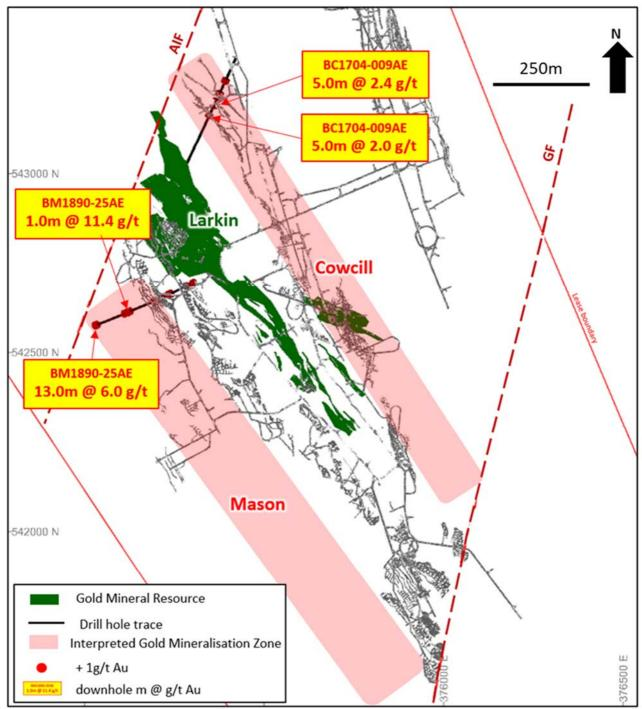
Figure 10-5 Beta Hunt plan view highlighting recent significant gold results from Mason and Cowcill drilling (Karora news release August 23, 2022)
