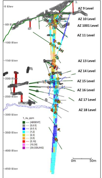
Figure 14-16 A Zone model (undepleted) and drill hole grades, cross-section (2) looking north
