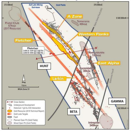
Figure 7-5 Plan view of 2020 gold resources and interpreted gold shear zone targets Source: Karora
