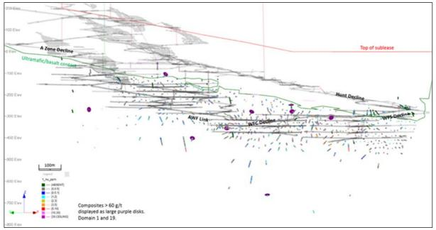
Figure 14-5 Western Flanks (Domain 8) composite data, long section looking east
