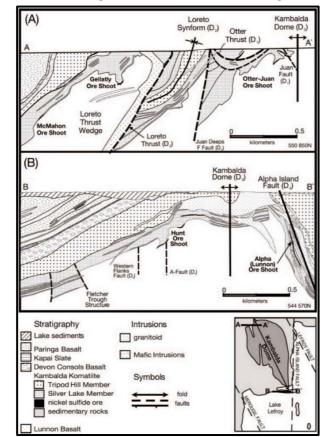
Figure 7-4 Schematic cross-section through the Kambalda Dome looking north Source: Stone et al. (2005)
