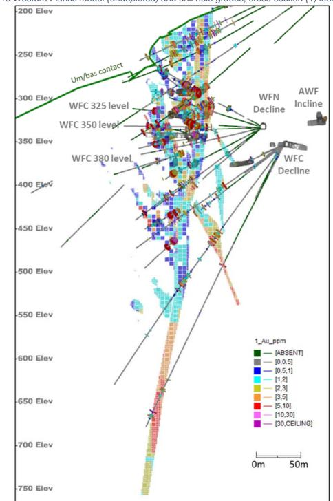
Figure 14-15 Western Flanks model (undepleted) and drill hole grades, cross-section (1) looking north
