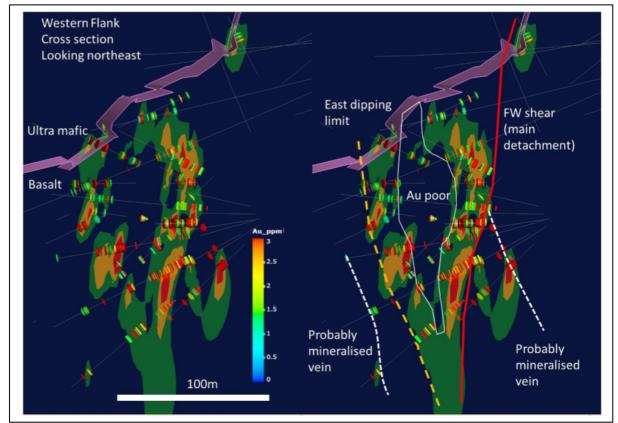
Using isosurfaces from a Leapfrog model, the study identified an apparent steep plunge orientation to the northwest (Figure 7-12). This interpretation is supported by structural measurements on a major cross-cutting fault which showed the dominant movement was steep from the northwest.
