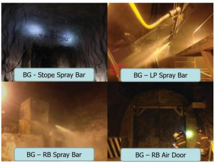
Figure 8: Typical dust controls
