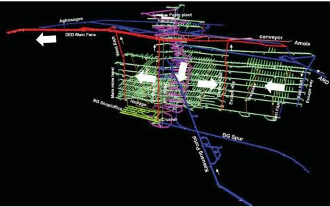
Figure 6: Big Gossan mine ventilation schematic
