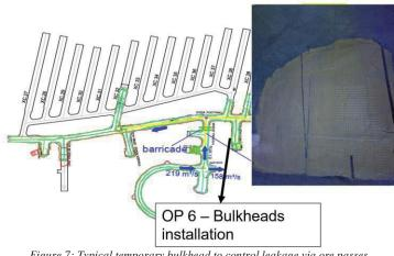
Figure 7: Typical temporary bulkhead to control leakage via ore passes
