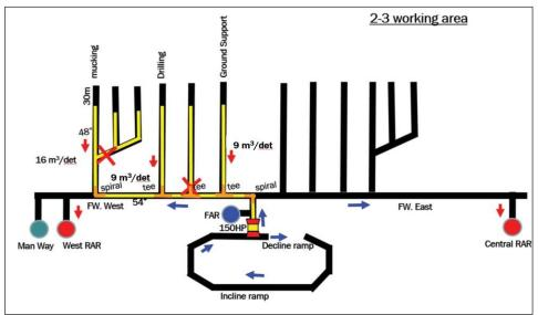
Figure 5: working area based on single auxiliary fan 150HP Capacity
