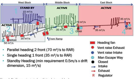
Figure 4: Big Gossan mine typical ventilation design each level
