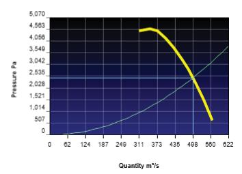
Figure 6: Big gossan main fan operating point
