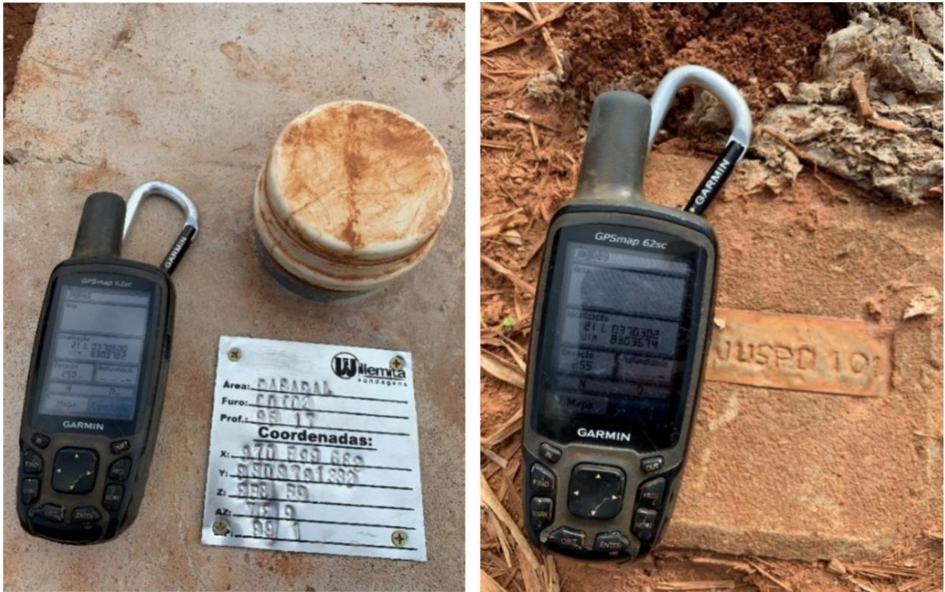
Figure 12-1: Drill Hole Location Quick Check Procedure.
