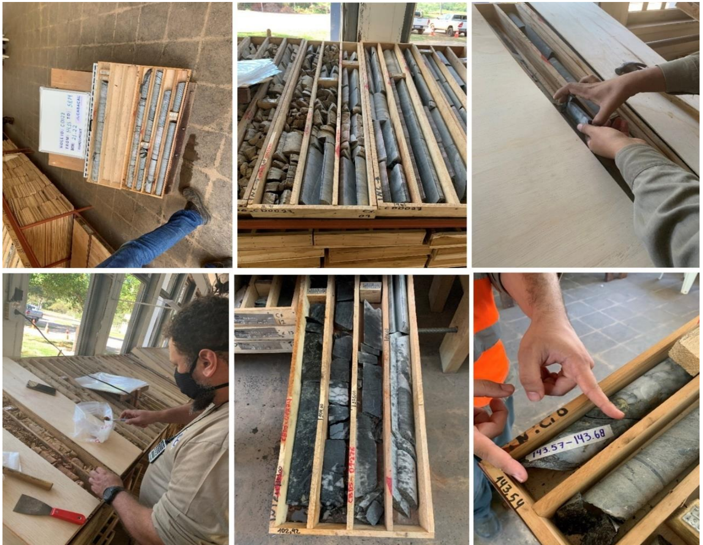
Figure 10-4: Examples of The Drillhole Procedures Implemented on Cabaçal Project
