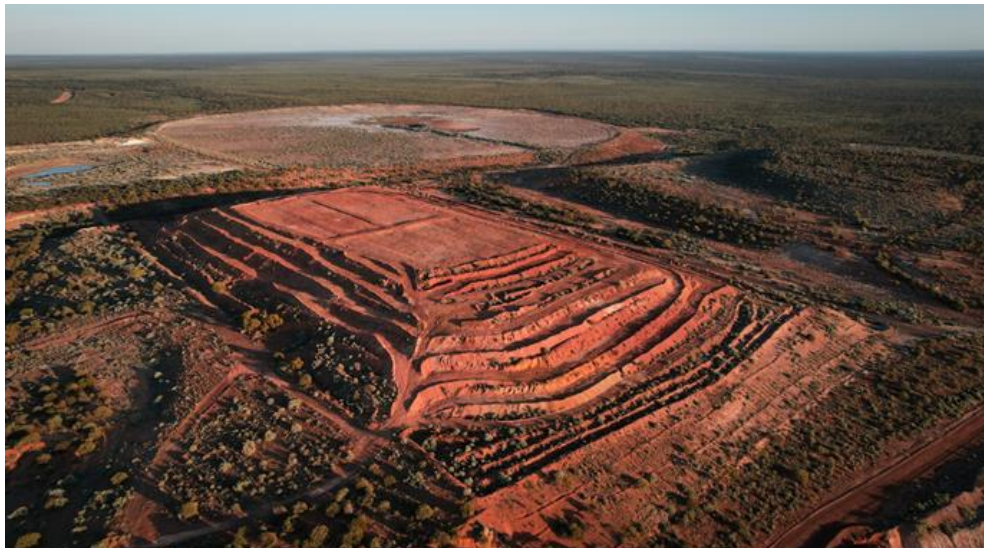
MGGP heap leach dump.
