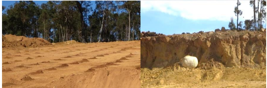
Left: Blastholes on Hardcap after sheeting with low grade. Right: Hardcap (hard brown) Friable (soft yellow), relict fresh remnant Dolerite dyke boulder
