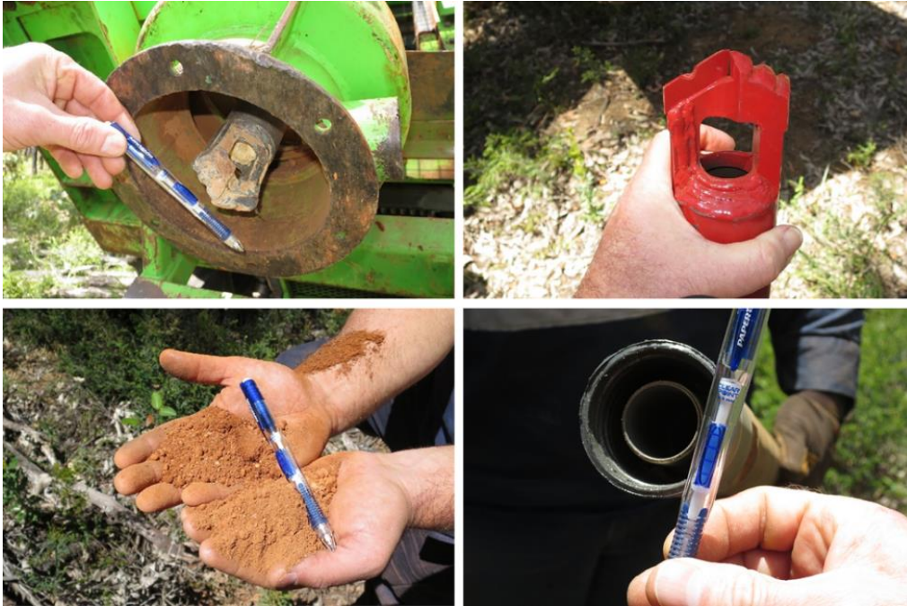
Figure 7-4: Drill Bits, Reverse Circulation Drill String and Particle Size of the Sample Residue (SLR, 2021) Scale pen diameter 13 mm
