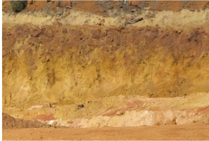
Figure 12-1: Undulating Hanging Wall Hardcap Surface; and Footwall (white clay, lower right in the floor) (Left: Pearman, 2015 & Right: SLR, 2021)
