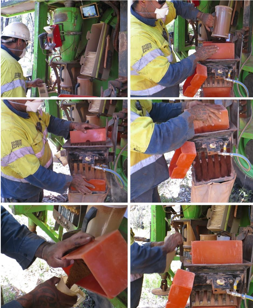
Figure 7-5: Sample Catching and Riffle Splitting Practices (SLR, 2021)
