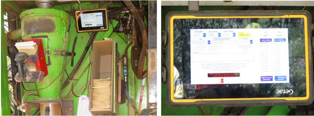
Figure 7-6: Barcode Reader and Digital Recorder Mounted on the Drill Rig (SLR, 2021)
