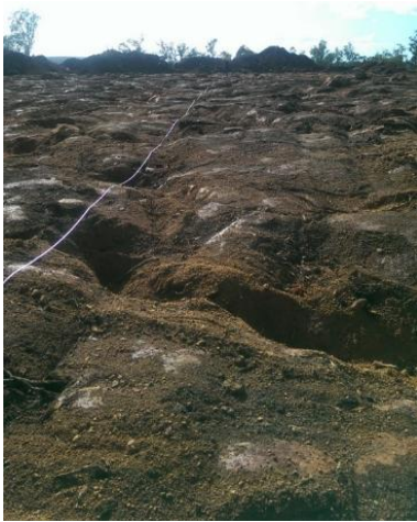
Figure 12-1: Undulating Hanging Wall Hardcap Surface; and Footwall (white clay, lower right in the floor) (Left: Pearman, 2015 & Right: SLR, 2021)
