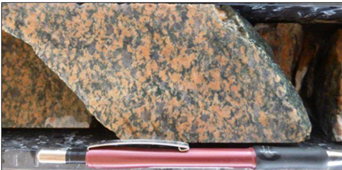
Figure 7.2.3 Distal Alteration: Haematite-Chlorite Pervasive Alteration (from Direct Footwall of Mineralisation at Souwa – DPRC0504 @ 157 m Depth) (Source: Centamin, 2021)
