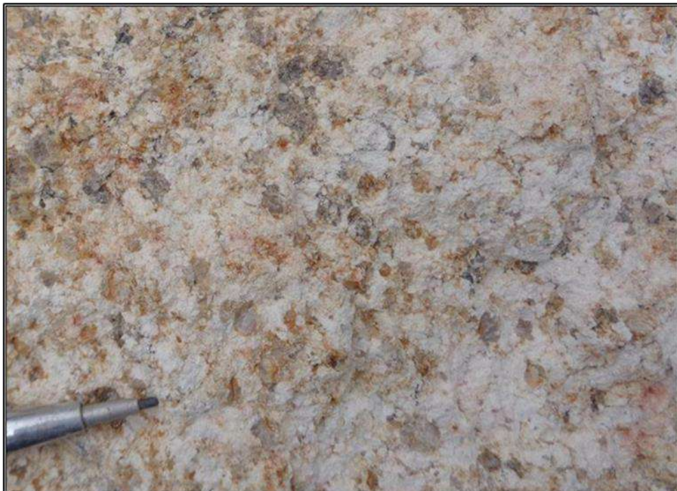
Figure 7.2.7 Saprock (Original Fabric and Mineralogy is Partially Preserved) (Source: Centamin, 2021)
