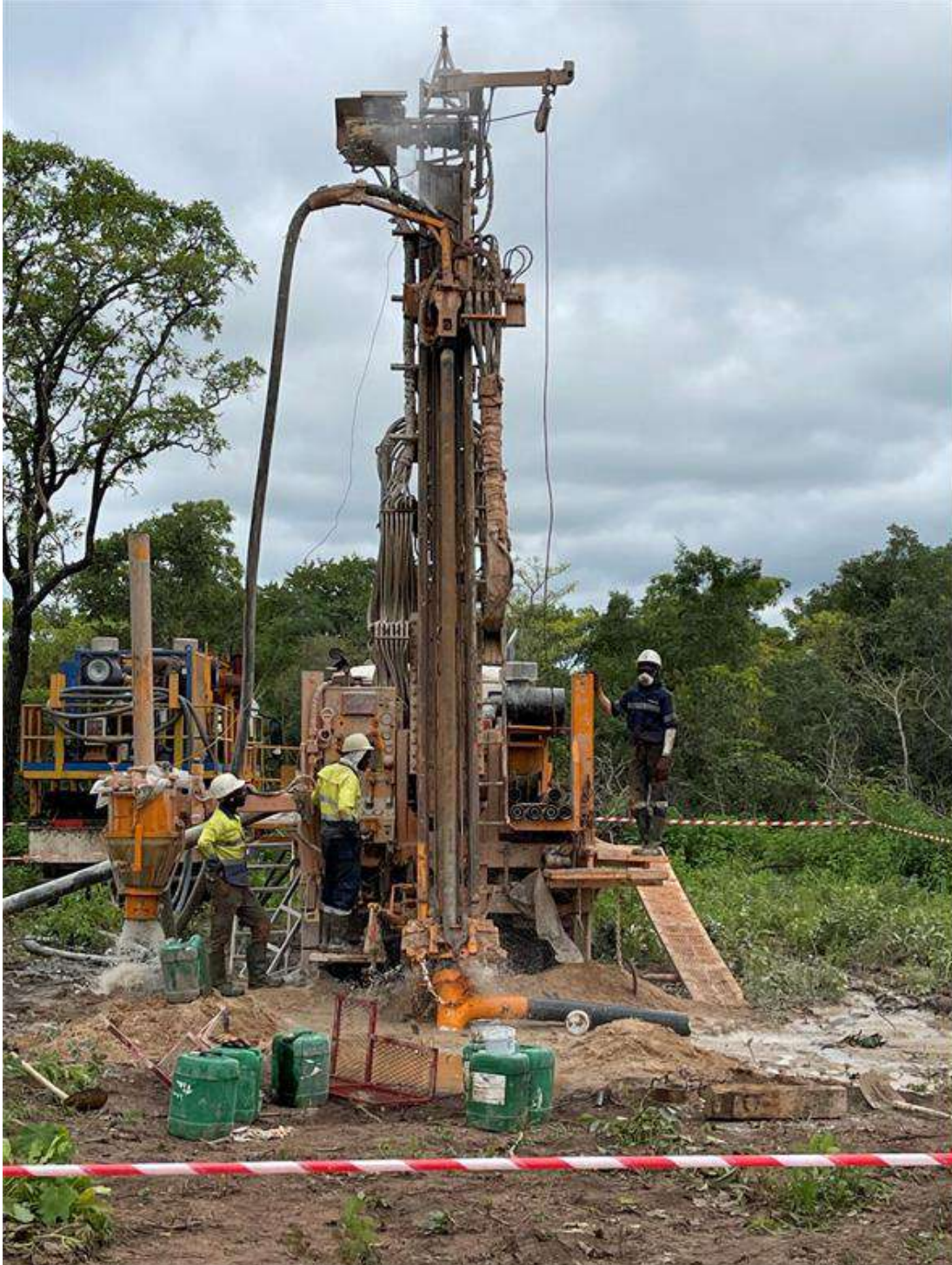
Figure 10.1.1 The Geodrill UDR650 Multipurpose Drill Rig with Compressor Visible in the Background
