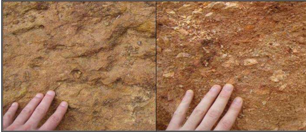
Figure 7.2.6 Two Examples of Doropo Saprolite Showing Quartz Vein Fragments in the Right Hand Photograph (Source: Centamin, 2021)
