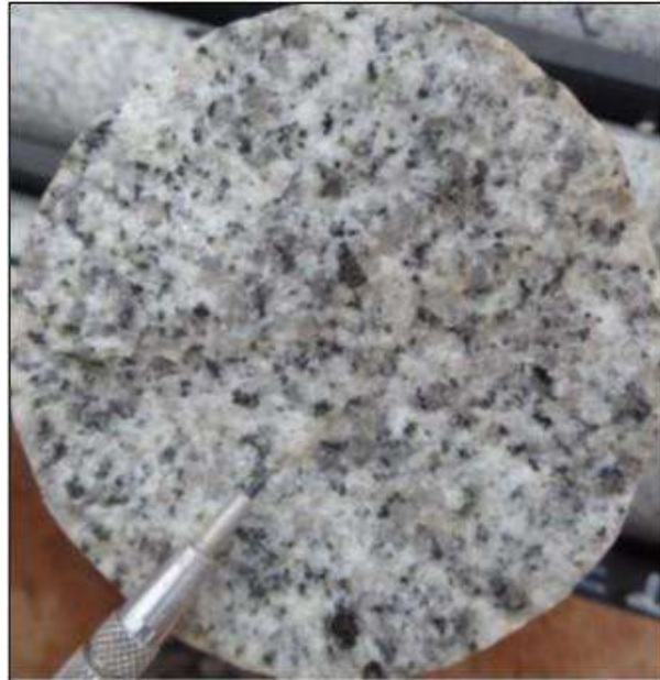
Figure 7.2.10 Fresh Granodiorite (Source: Centamin, 2021)
