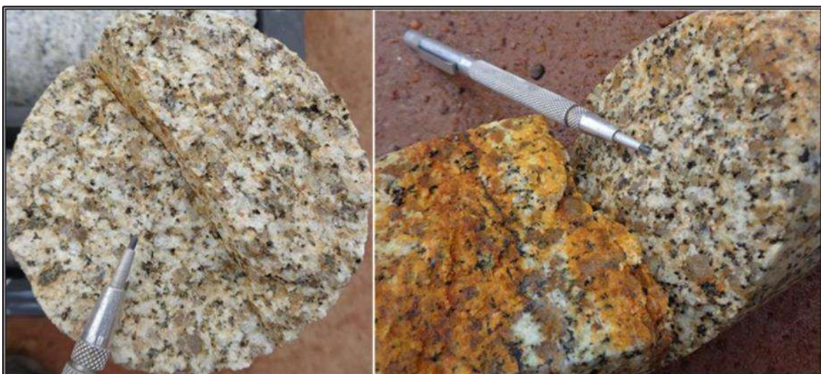
Figure 7.2.9 Transition Zone Between Lower Saprolite and Fresh ROCK (Source: Centamin, 2021)
