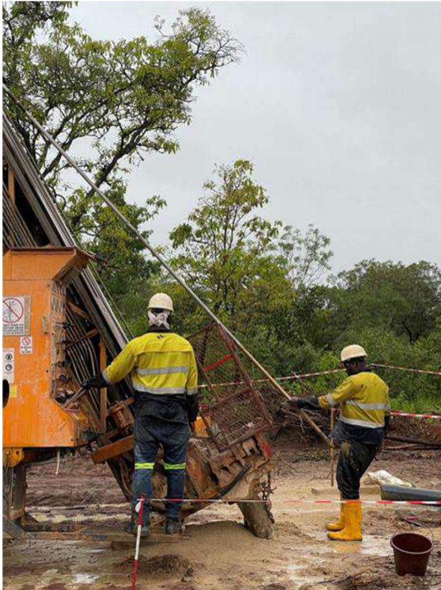
Figure 10.4.1 The Reflex EZ Shot Tool About to be Inserted into a Drill Hole to Take a Downhole Survey Reading
