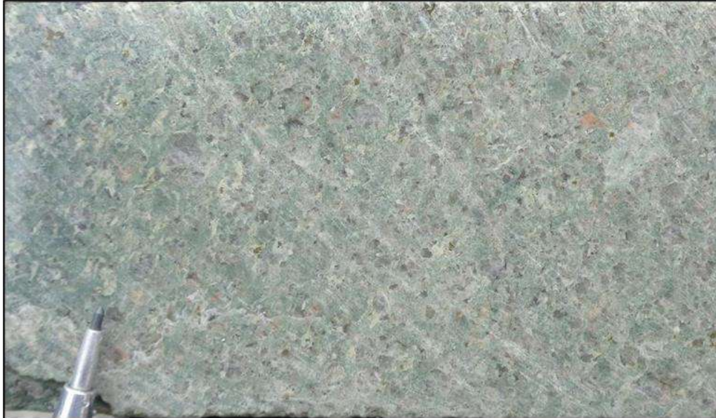
Figure 7.2.4 Proximal Intense Sericite and Fine Grained Disseminated Pyrite Alteration (from the Han Deposit – DPRD0470 @ 94 m Depth) (Source: Centamin, 2021)
