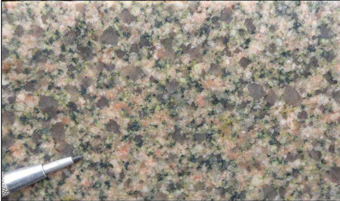
Figure 7.2.3 Distal Alteration: Haematite-Chlorite Pervasive Alteration (from Direct Footwall of Mineralisation at Souwa – DPRC0504 @ 157 m Depth) (Source: Centamin, 2021)
