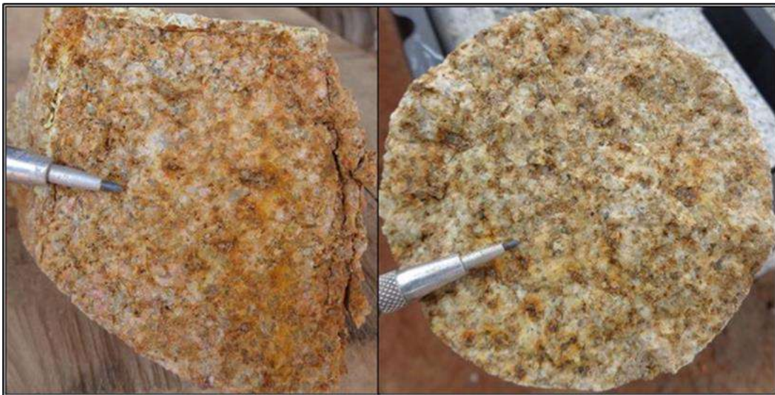
Figure 7.2.8 Saprock (Source: Centamin, 2021)
