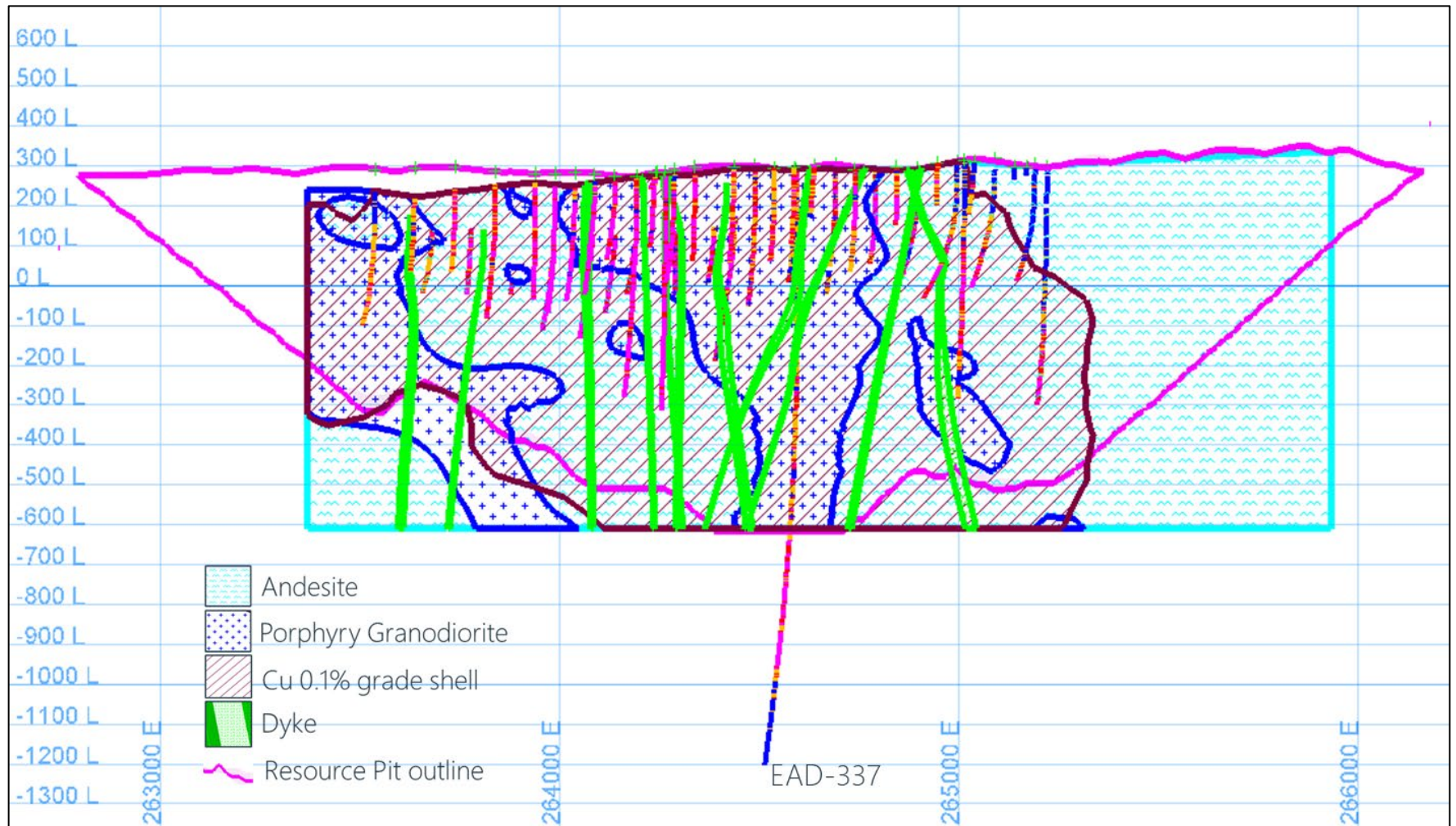
Figure 6-6: Geological Cross-Section Showing Copper Grade Shell (N 3103350)
