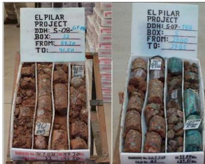
Figure 6-8: Typical Qwu Core Samples – (note large, mineralized breccia fragments)
