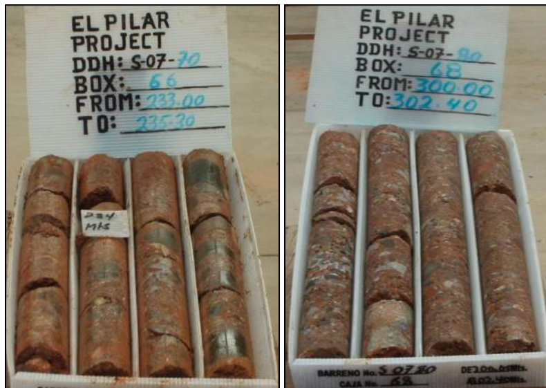
Figure 6-6: Typical Qwl Core Samples - Calcite Cemented Debris Flow Deposit with Volcanic Fragments
