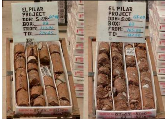
Figure 6-7: Typical Qwt Core Samples - (note red-brown color and angular fragments of volcanic rocks)
