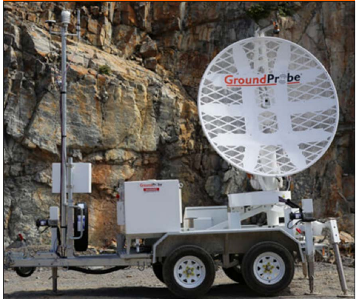
GroundProbe monitoring radar deployed at site
