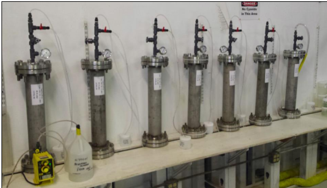
Figure 13-5: Series Leach Test Apparatus
