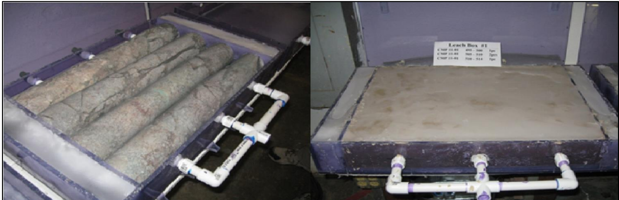
Figure 13-1: Leach Box Setup with Core Sample (Left) and Loaded with Silica Sand (Right)
