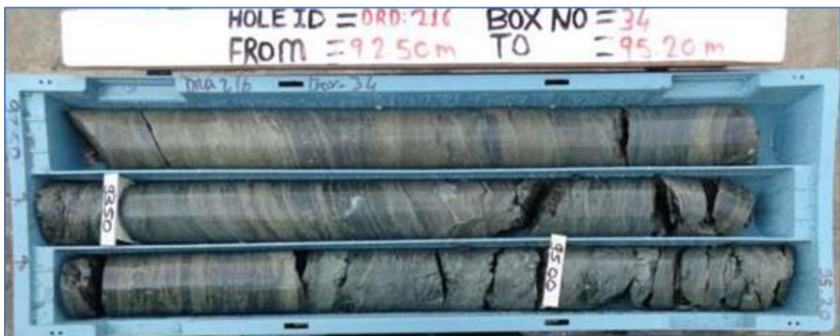
Figure 7-22: Chlorite-Sericite Schist with Pyrite Veining in Drill Core
