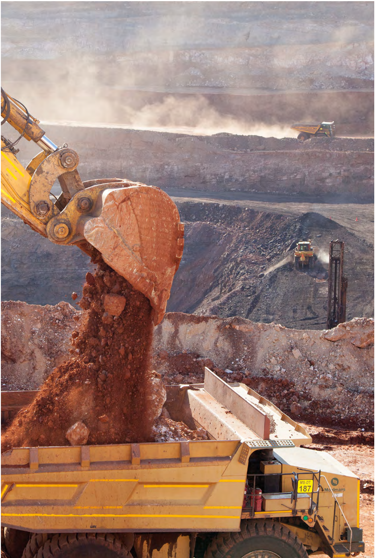
Waste stripping at the Tshipi Borwa mine.
