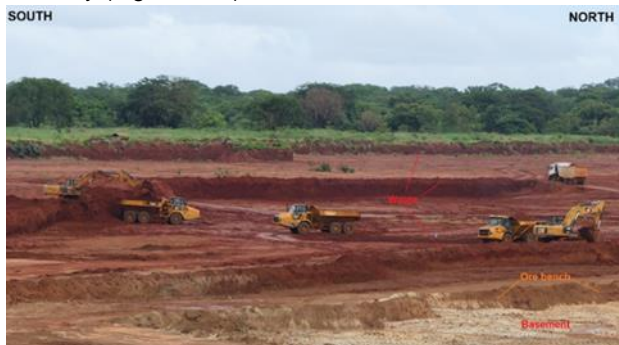
Figure M11: Systematic and selective mining under Geology supervision
