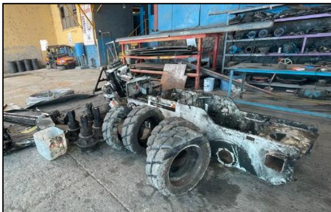
(StopeMate pneumatic long hole drill in disrepair, discovered at VMC)
