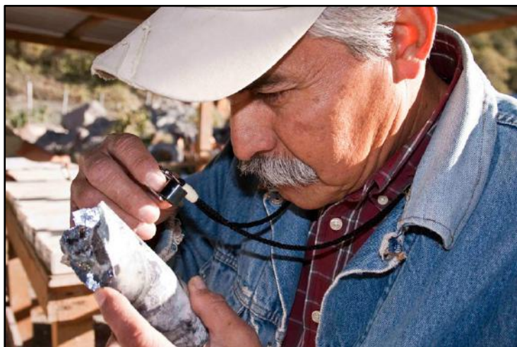
(Claudio Conseco, geologist at Topia, checking drill core at the core shack facilities)
