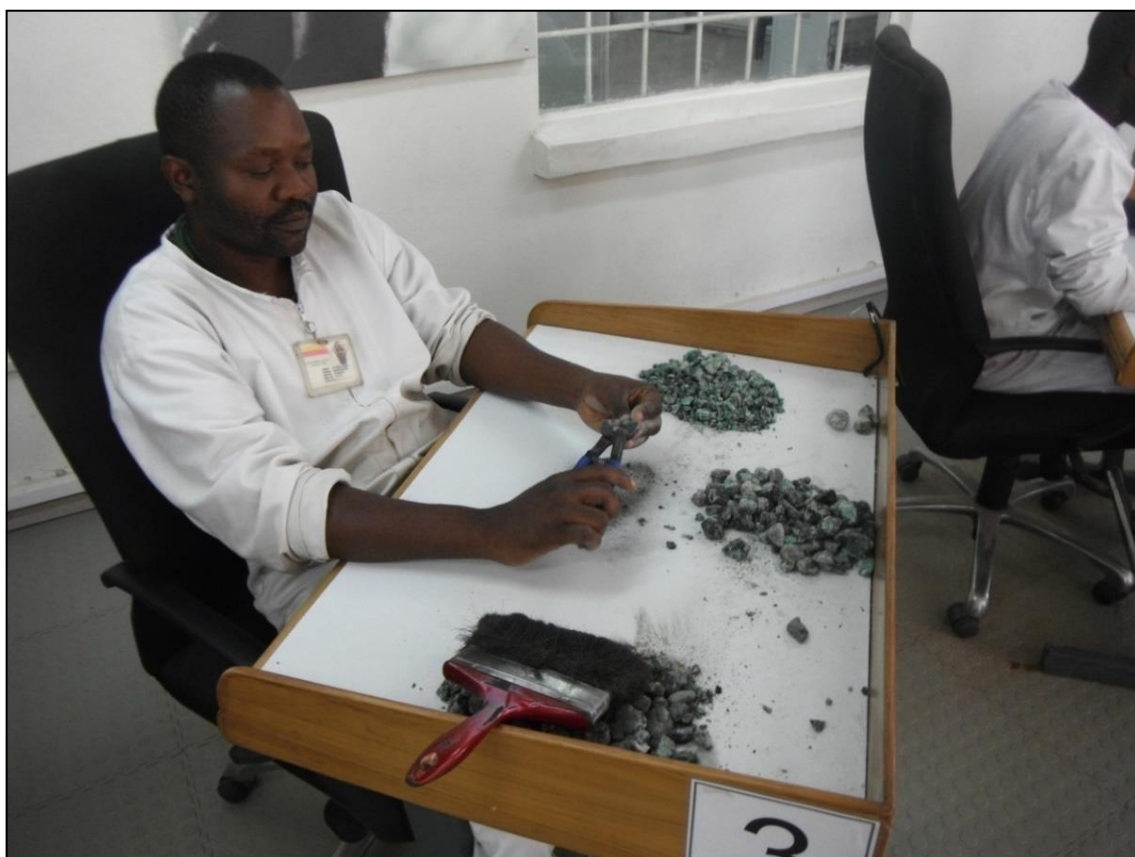
Figure 2-17: Kagem Sort House Worker “Cobbing” Host Rock from Emerald Gemstones
