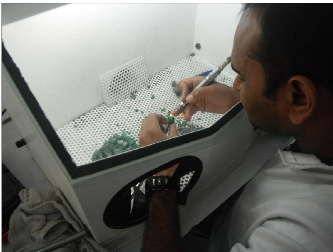
Figure 2-18: Kagem: Sort House Worker Removing Waste Material from a High Quality Emerald
