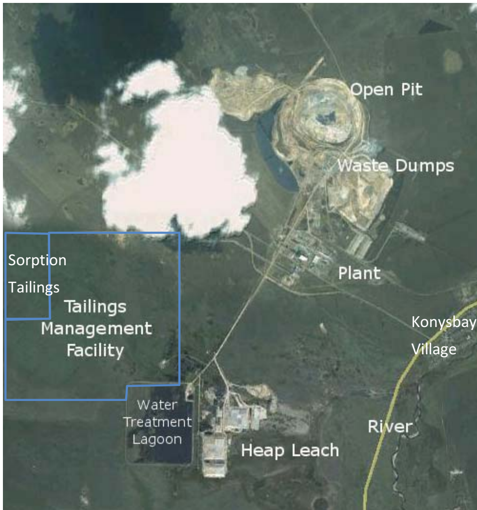
Photo 3.3: Aerial View Showing Location of Main Mine Components. The Outline of the new TMF is shown approximately
