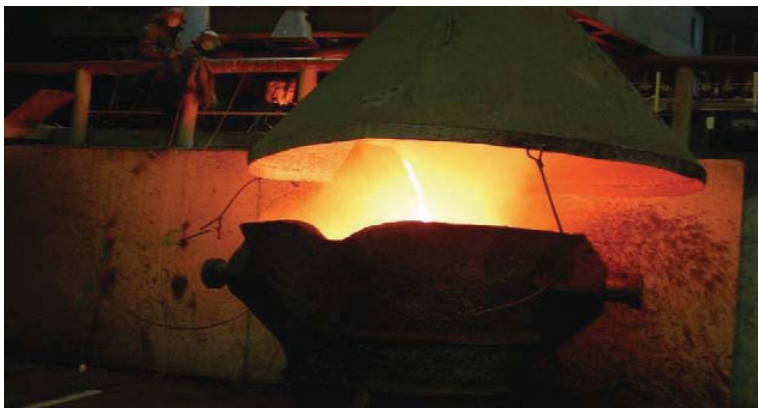
Photo 16.1: Tapping Lead Bullion from Lead Blast Furnace
