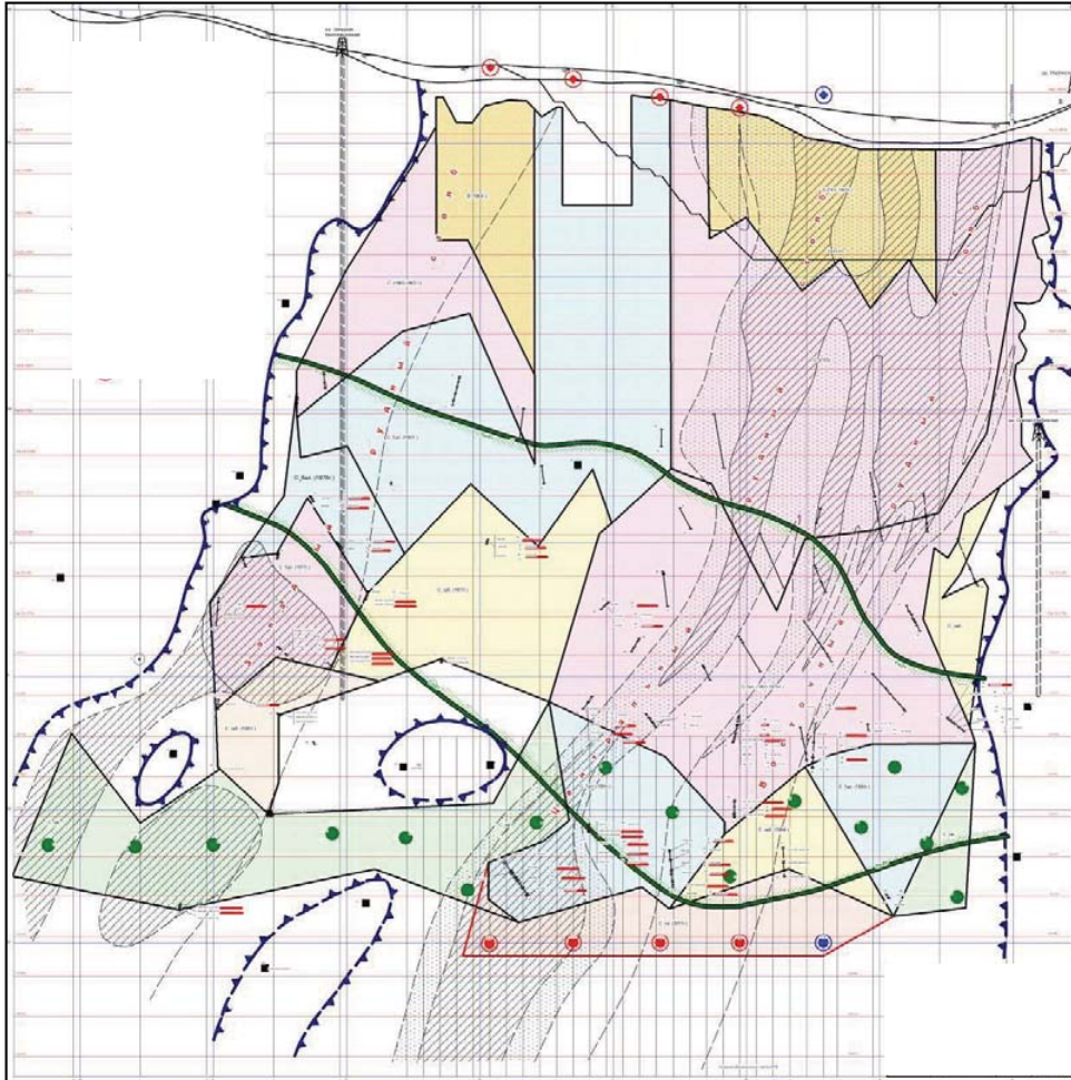
Figure 9.5: Long Section showing Location of Deep Horizon (Collars and targets shown in red) and Flank (targets shown in green) Exploration Drill holes (Grid:200m)
