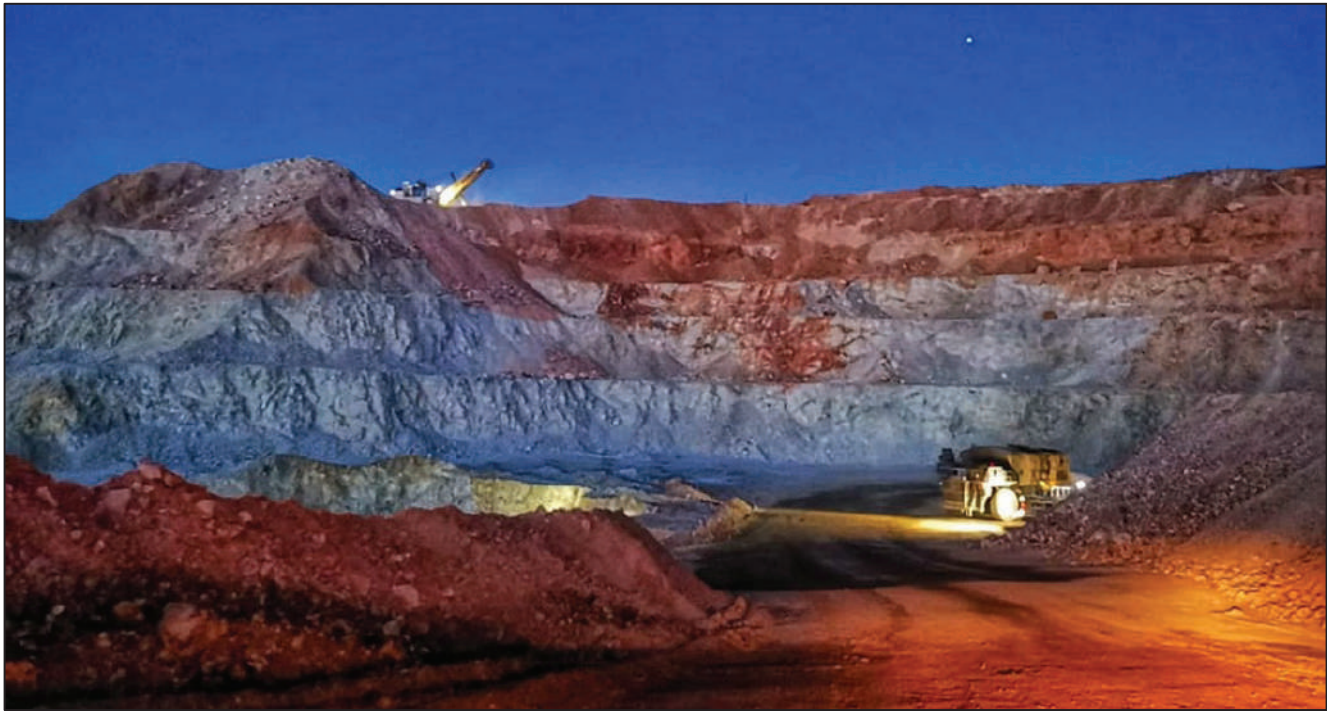
Figure 6.5: Oxidation Zone (Red) and Supergene Zone (White) in the Western Part of the La Caridad Pit
