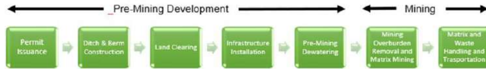
Figure 13-1: Dragline Mining Process
