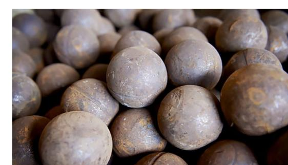
Forged steel balls, known as media, are used within the mills to break down the ore. The steel balls are designed to break down while progressively reducing the size of the rock.
