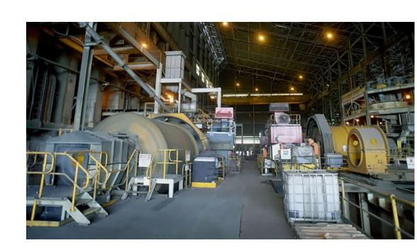
To separate the copper from the other minerals and waste, the ore is finely grinded within the SAG and Ball Mills, then a flotation process is used to 'concentrate' copper into a product that can be fed to the Copper Smelter.
