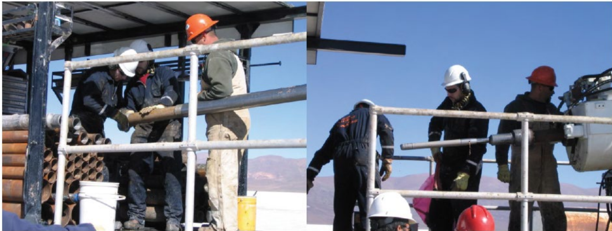
Figure 9.5: Recovery of the lexan core and split spoon samples on the sonic
