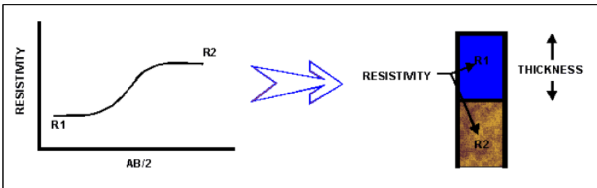
Figure 9.7: The process of converting field resistivity measurements to interpretation of thickness and resistivity
