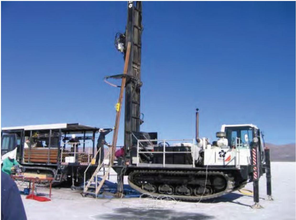
Figure 9.4: Sonic drilling rig operating at Olaroz in 2010
