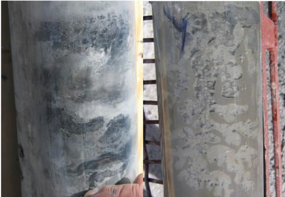
Figure 7.4: Clay material in Unit UH 1, showing bioturbated clayey sediments (from Houston and Gunn, 2011)
