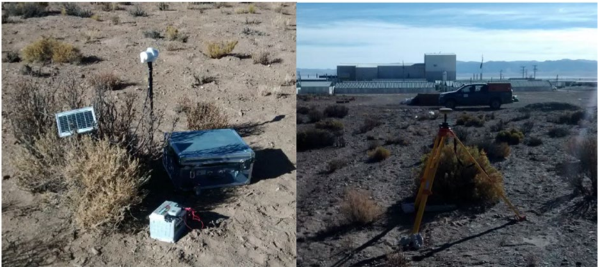
Figure 9.10: Installation of the magnetic base station (left) and the GPS base station (right)
