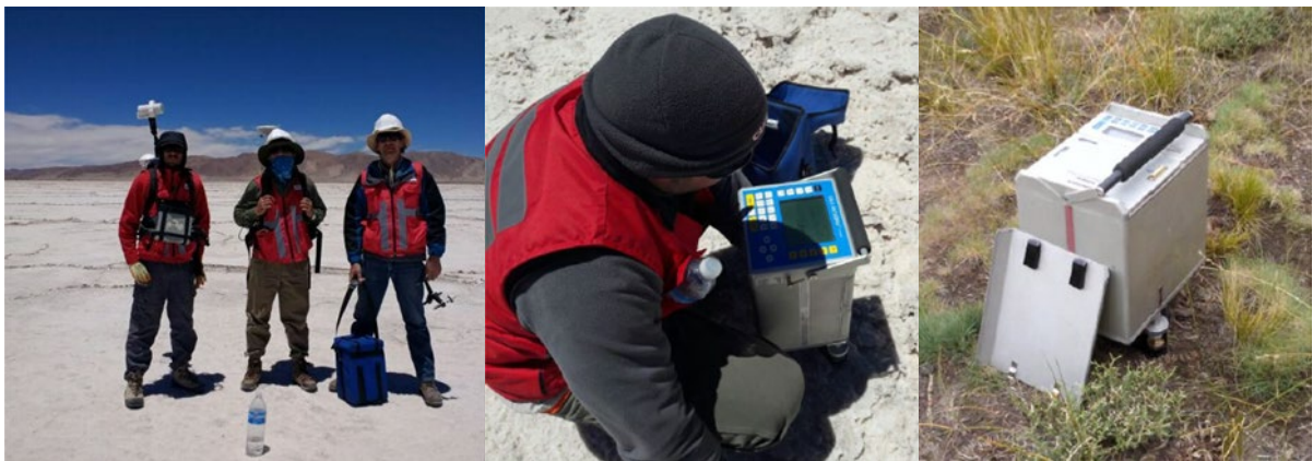
Figure 9.9: Team conducting ground magnetic survey, Scintrex CG5 unit and Scintrex CG3 unit
