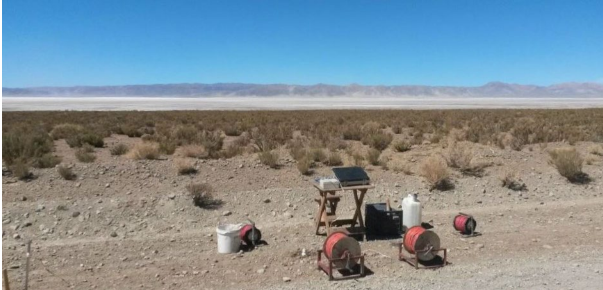
Figure 9.6: SEV geophysical equipment in use in the Archibarca area
