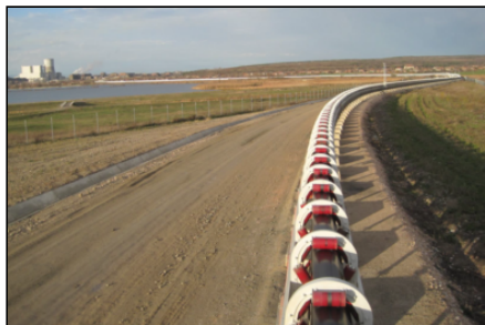
TAKRAF’s Automatic Belt Training System (ABTS) to control tube conveyor rotation & overlap
