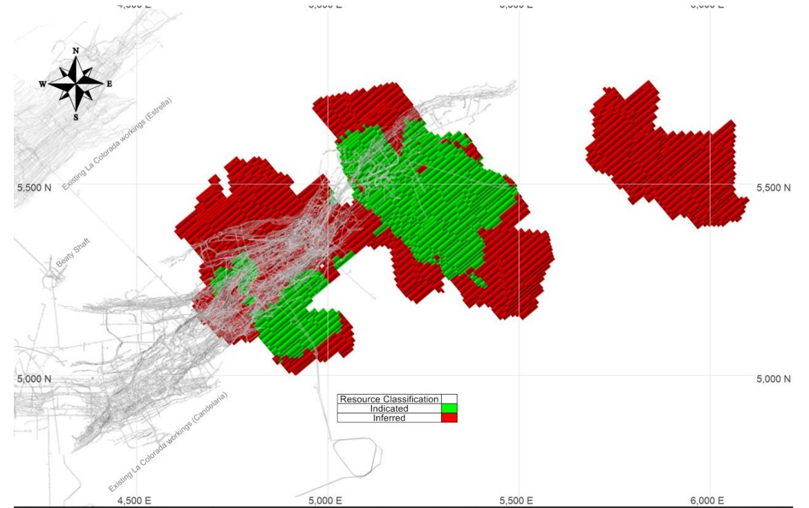
Date: 13 September 2022 | Plan view with existing workings | Mine Coords La Colorada Skarn Mineral Resource Classification Figure 2
