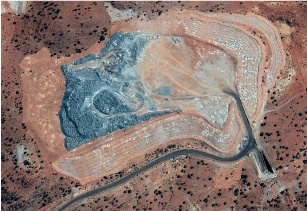
Plate 4 Aerial view of the Potosi WRE (January 2019) following reprofiling and contour ripping of batters
