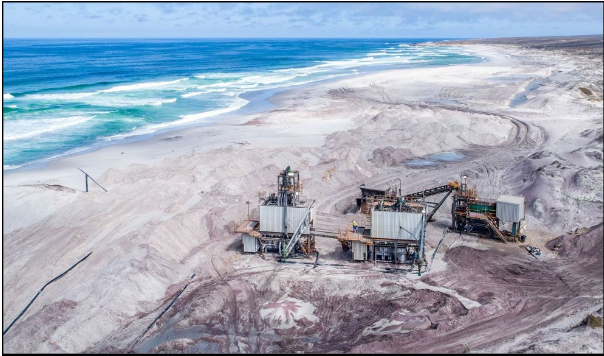
Figure 4 – Overview of mining operation and primary concentrator at beach 10 of the Northern Beaches
