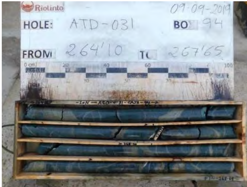
Figure 10-7: Photographic record of the core boxes after delivery. Core is HQ diameter (Atalaya, 2019).
