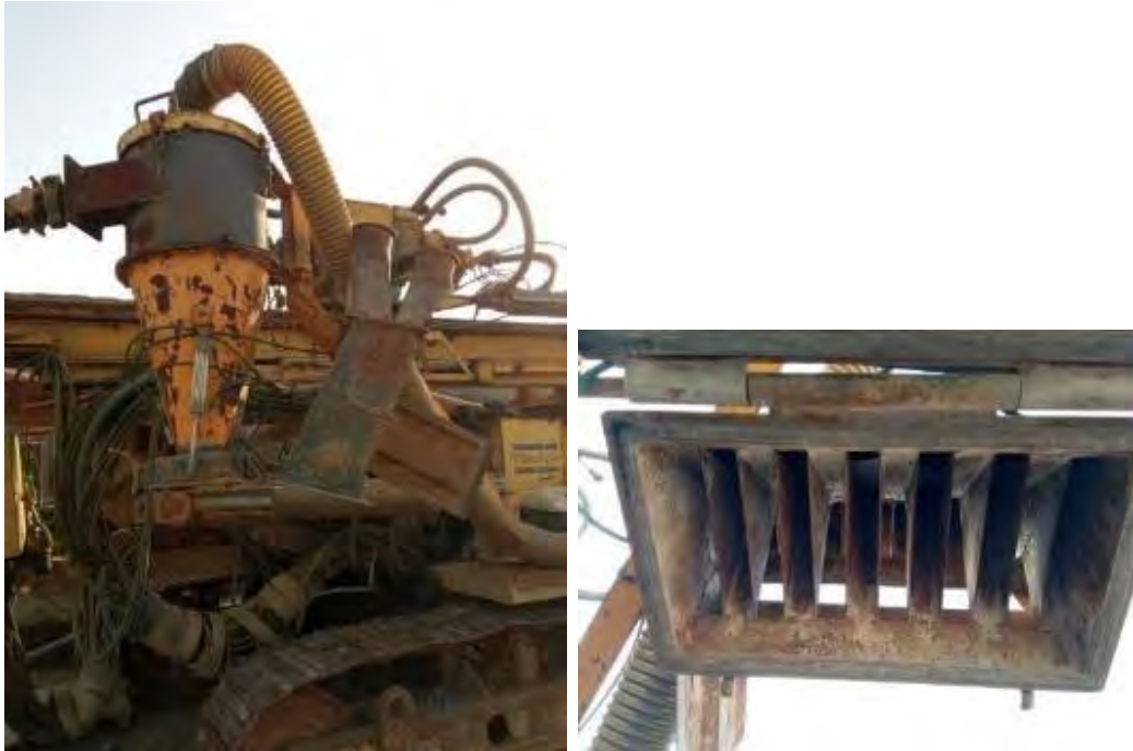
Figure 11-6: RC rig sample splitter (Atalaya, 2022).
