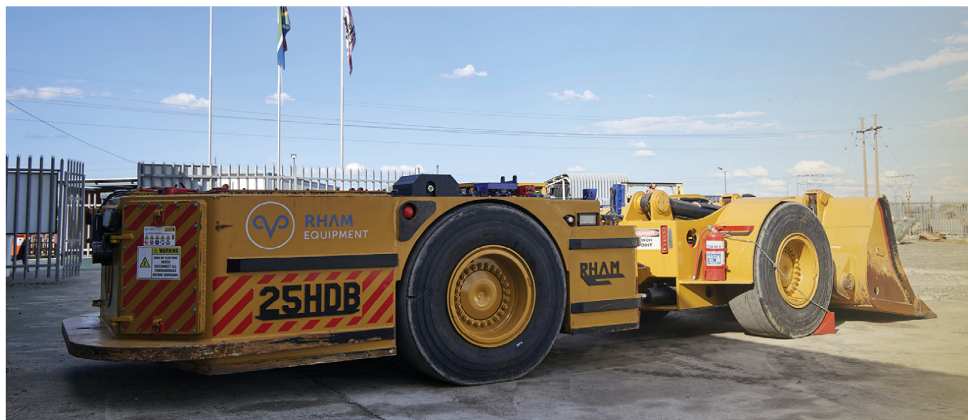
Remotely operated battery-electric LHD at the Bathopele operation at SA PGM
