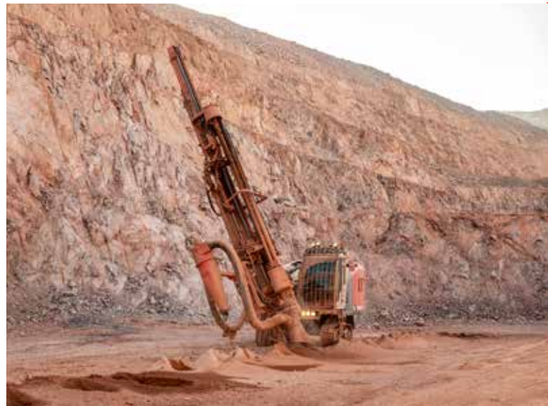
Two Leopard DI650i intelligent down-the-hole (DTH) drill rigs are put to work at the open-pit gold mine La Herradura. The site also employs two Leopard DI550 DTH drill rigs (above).
