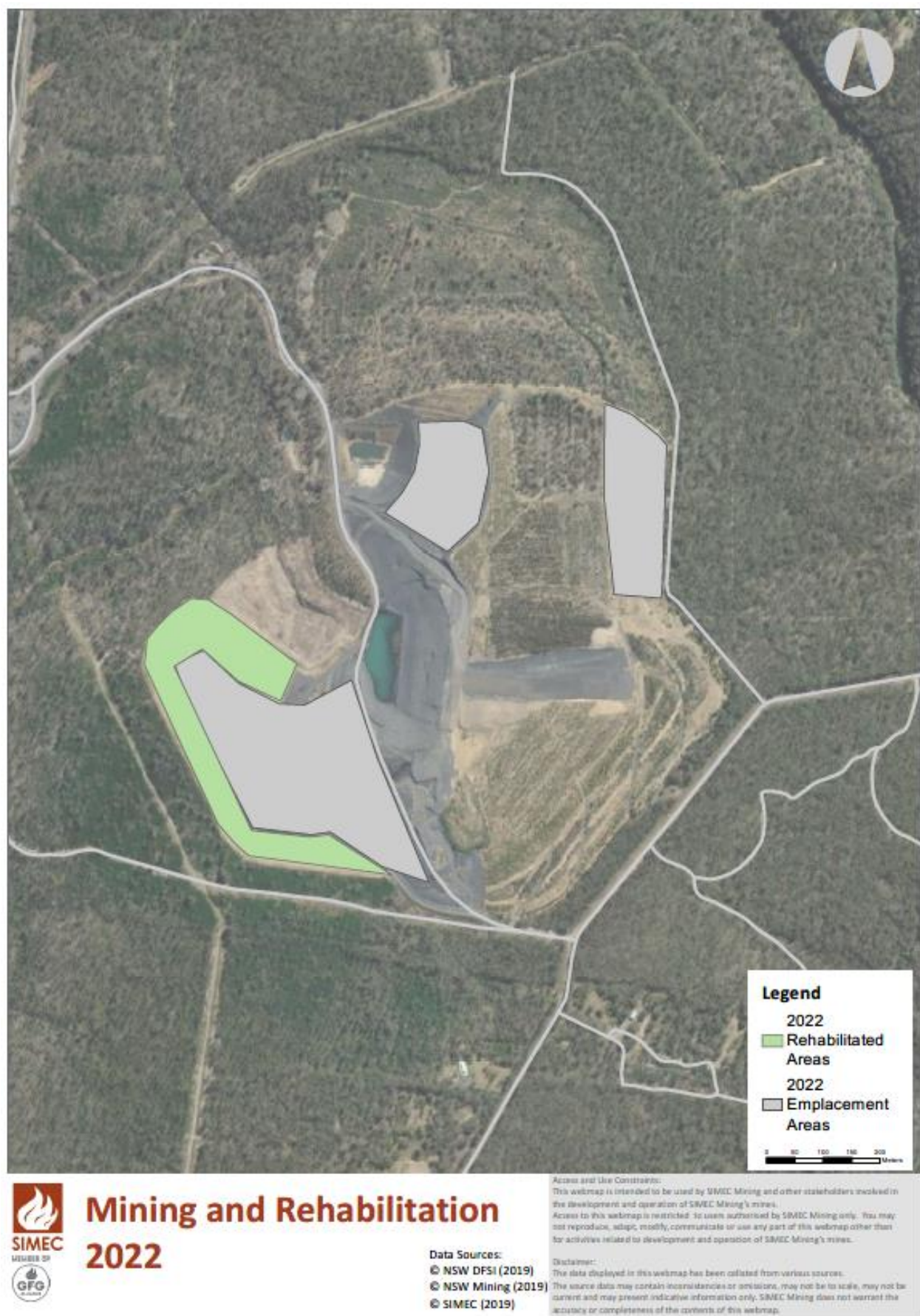
Figure 52 Reject Emplacement Areas and completed Rehabilitation works during 2022.
