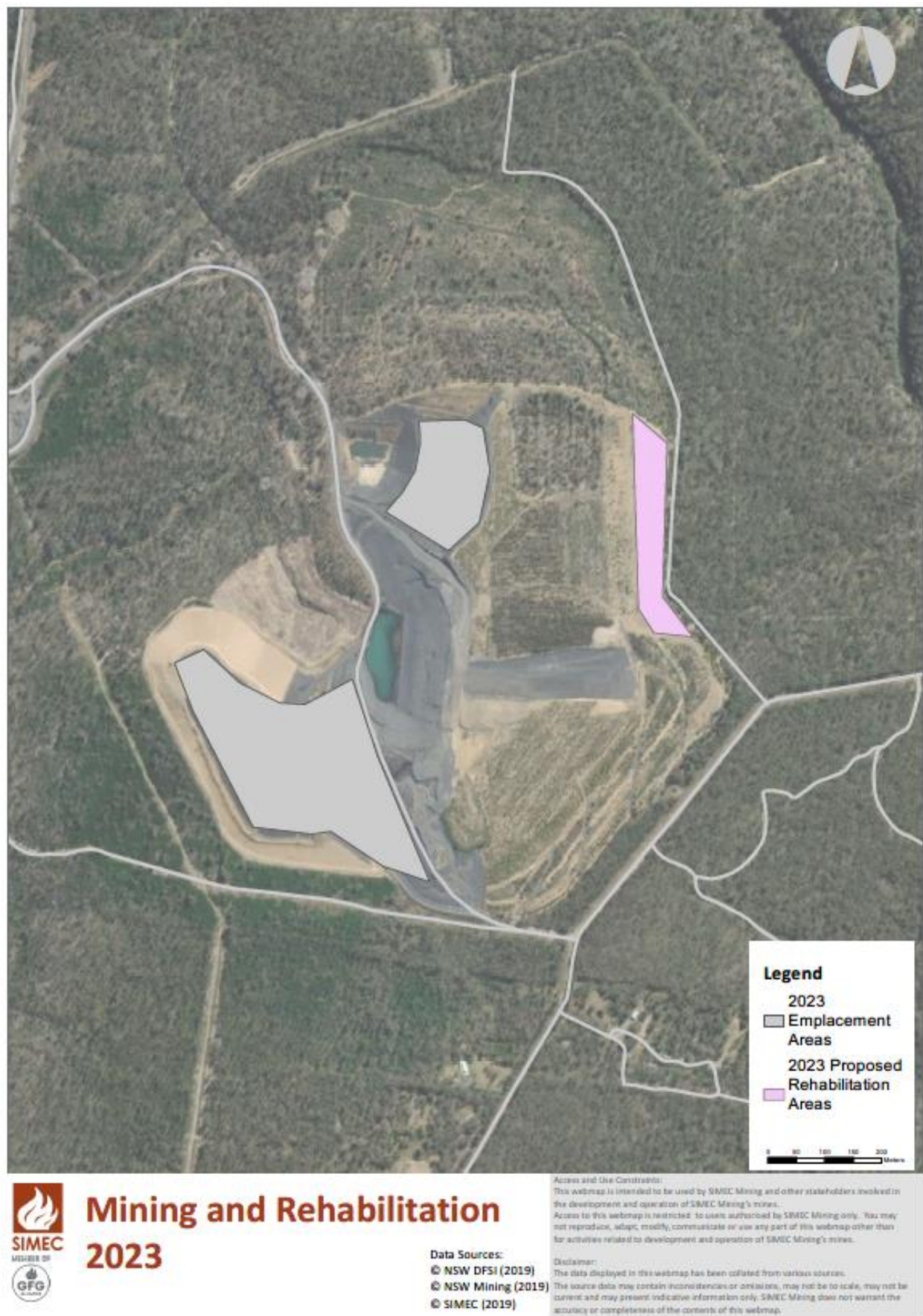
Figure 53. Reject Emplacement Areas and proposed Rehabilitation works for 2023.
