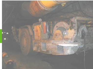
That's the new 2-yard electric scooptram, now in operation at Creighton mine. A new concept in load-haul-dump operation, the unit is operating in a cut-and-fill stoping complex on the 6600 level.
