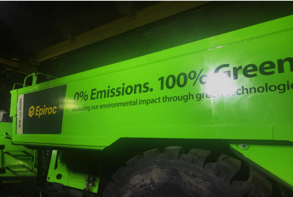
Photo: Battery electric haul-truck at Creighton mine in Sudbury
