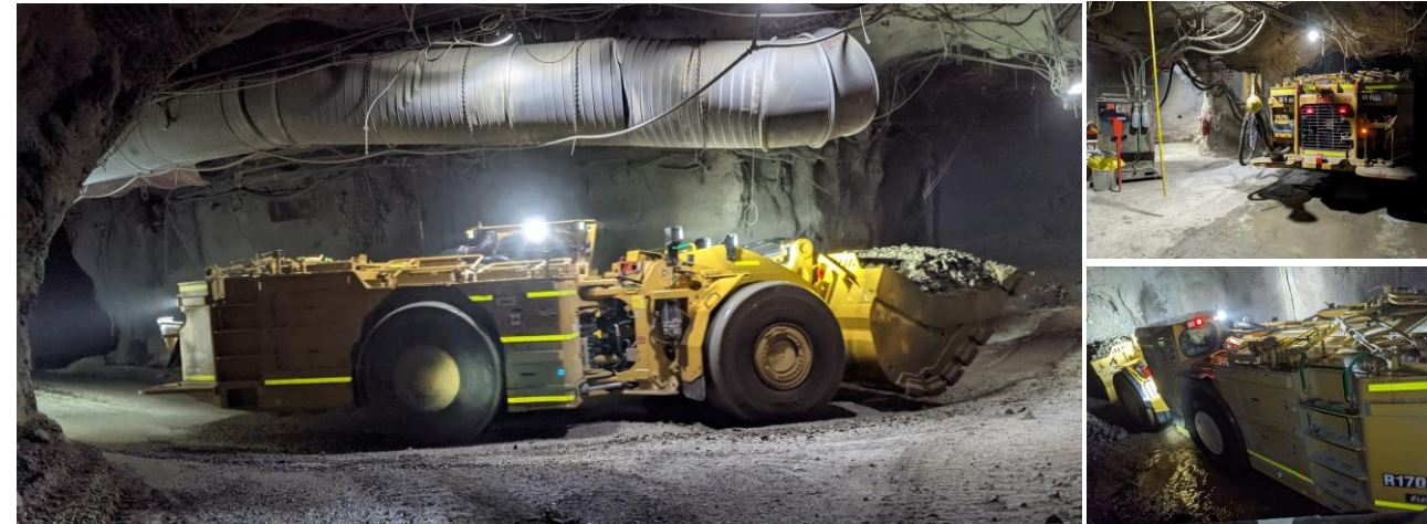
Photos: Battery electric LHD at Copper Cliff mine in Sudbury
