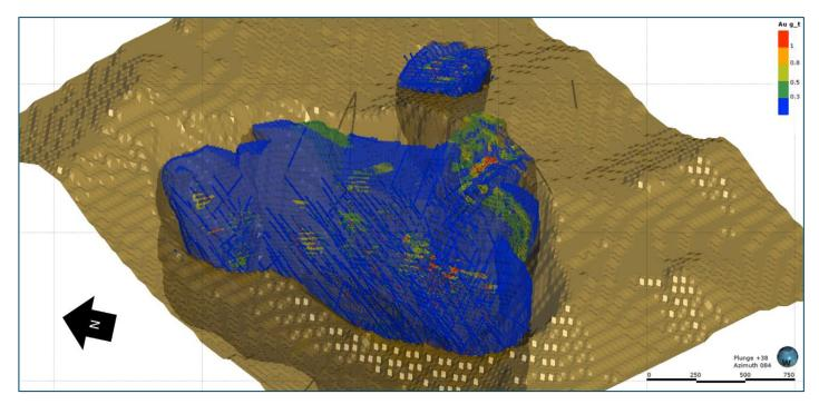
Figure 14-39: Isometric View of the Dorado Area Block Model and Base Case Optimized Pit Shell (Looking northeast)
