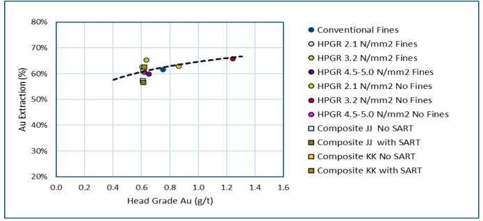
Figure 13-3: Impact of Process Variables on Recovery
