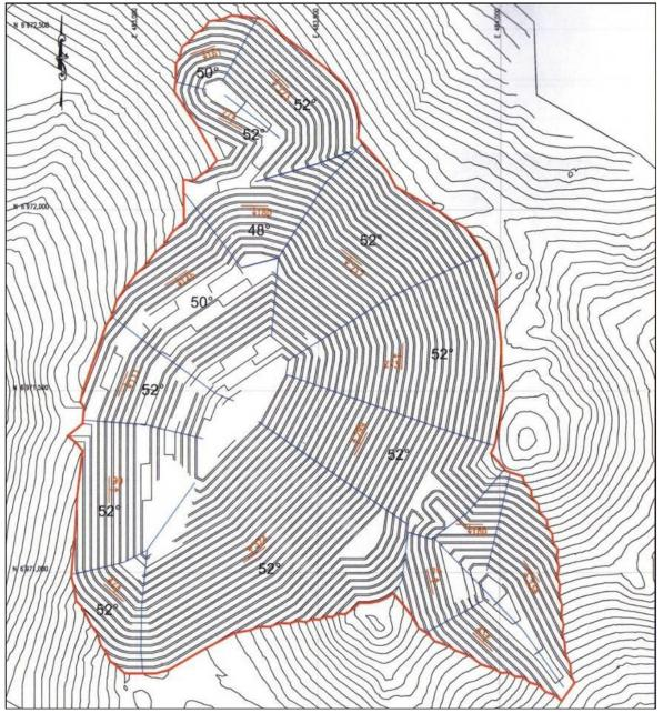
Figure 14-37: Preliminary Overall Wall Slope Sectors, Dorado Area Open Pits, Volcan Project
