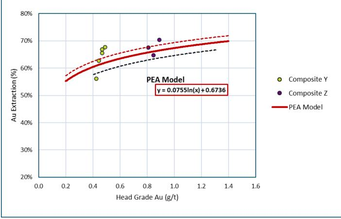
Figure 13-5: PEA Recovery Model – HPGR, 3.2 N/mm<sup>2</sup> pressure, fines retained
