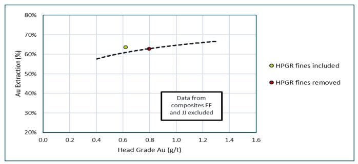
Figure 13-4: Impact of Fines Removal
