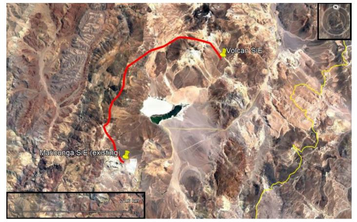
Figure 18-11: Proposed Transmission Line 110 kV route.
