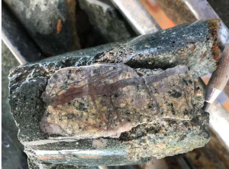
Figure 9.10 – IOCG/CRD Clast with A-type veins in Dacite Breccia in El Alacrán Deposit Drill Core Hole ASA-046
