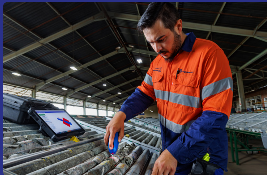
Photis Kalpakiotis (structural geologist) identifying orientation of structural faults in the drill core at Mogalakwena core yard
