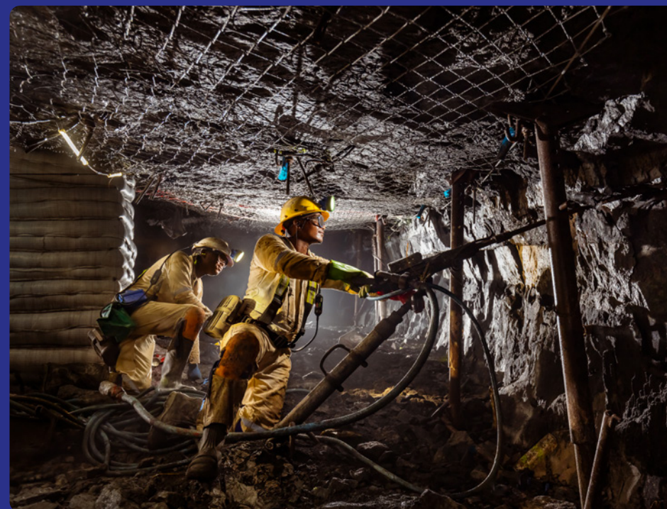
Drilling in a stope with blast-on-mesh at Amandelbult Dishaba
