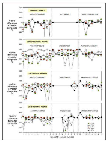
Figure 10-4: Variation of Metal Assays in Flotation Products
