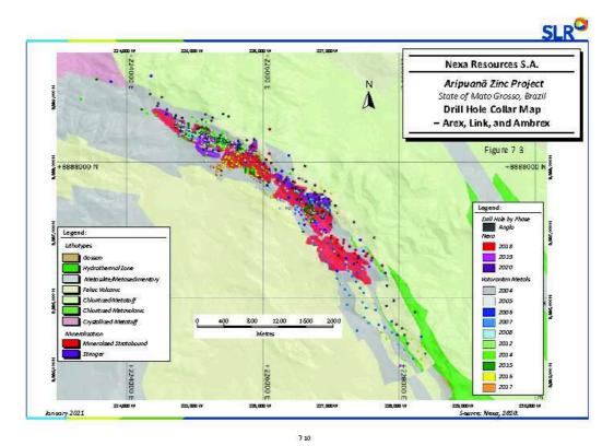
Figure 7-3: Drill Hole Collar Map – Arex, Link, and Ambrex
