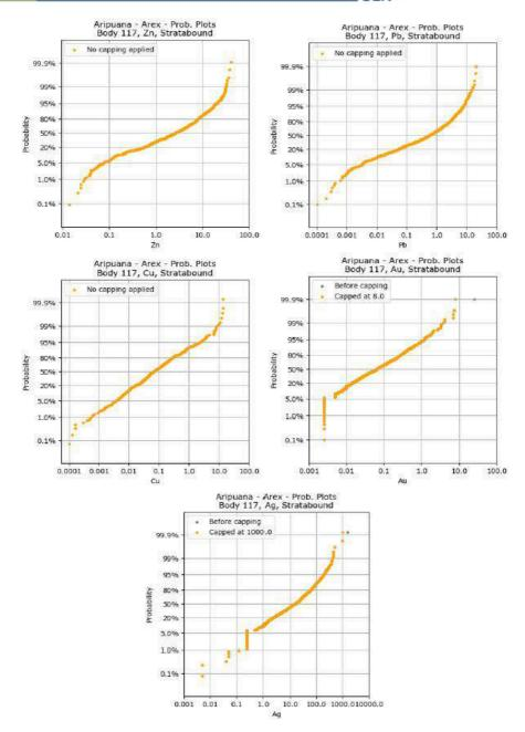
Figure 11-6: Capping Analysis for Body=117 (Arex)
