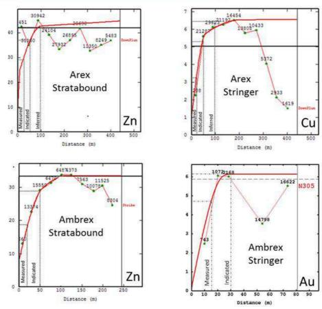
Figure 11-12: Global Variograms Used for Classification Criteria - Arex and Ambrex
