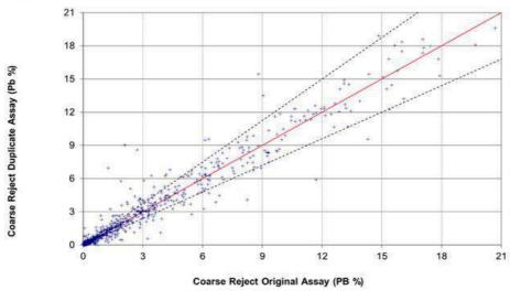
Figure 8-5: Analysis of Field Duplicate Data (Lead)
