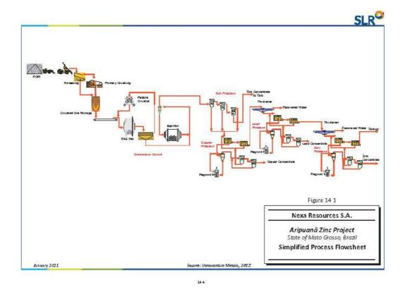
Figure 14-1: Simplified Process Flow Sheet
