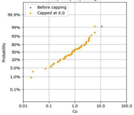
Figure 11-7: Cu Capping Analysis for Body=606 (Ambrex Stringer)
