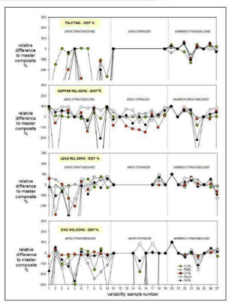
Figure 10-5: Variation of Metal Distribution in Flotation Products
