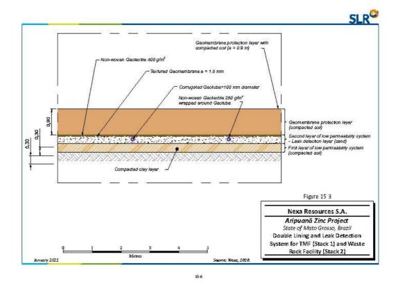
Figure 15-3: Double Lining and Leak Detection System for TMF (Stack 1) and Waste Rock Facility (Stack 2)
