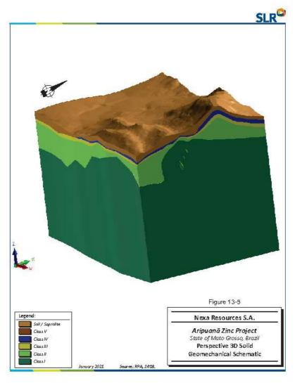
Figure 13-5: Perspective 3D Solid Geomechanical Schematic
