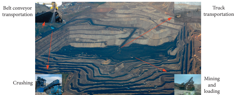
FIGURE 3: Schematic diagram of spatial layout of the coal mining semicontinuous process system.
